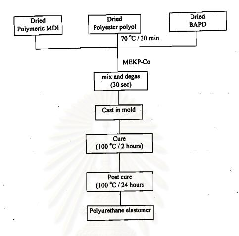
Scheme 2.2 Procedure for the preparation of polyurethane elastomer from MDI:Polyol:BAPD:MEKP-Co formulation
