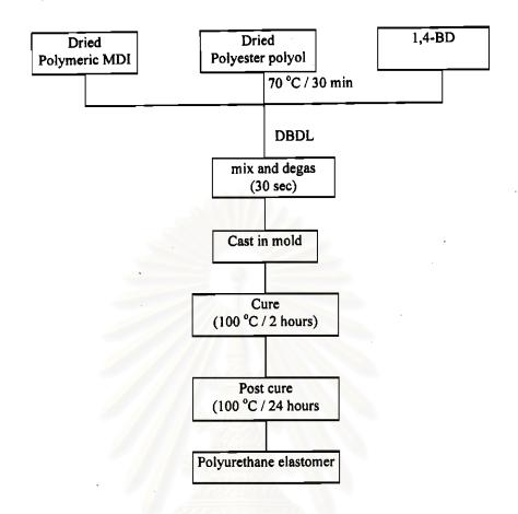
Scheme 2.1 Procedure for the preparation of polyurethane elastomer from MDI:Polyol:1,4-BD formulation
