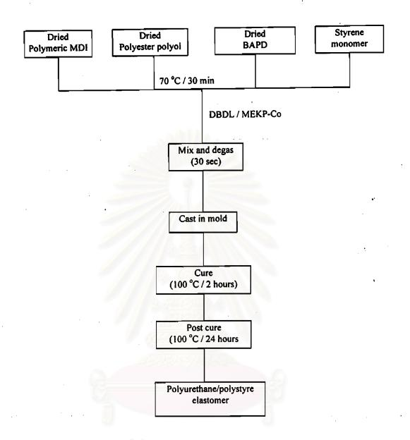
Scheme 2.3 Procedure for the preparation of polyurethane/polystyrene elastomers.
