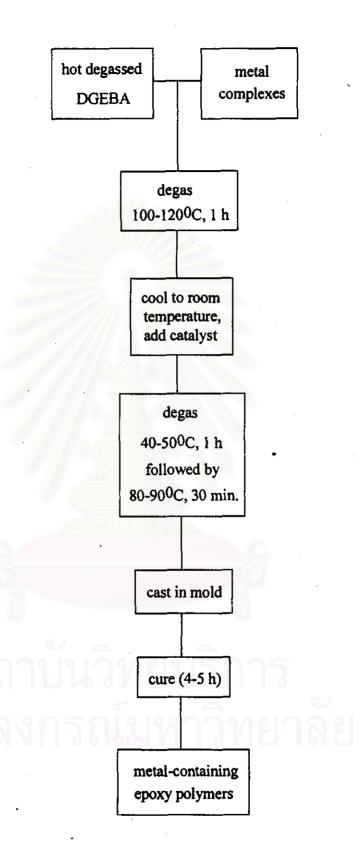
Scheme 2.1 The procedure for preparation of metal-containing epoxy
