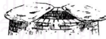
Stones to control draught.
