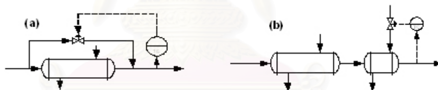
Figure 3.12: Control of P/P heat exchangers: (a) Use of bypass; (b) use of auxiliary utility exchanger.
