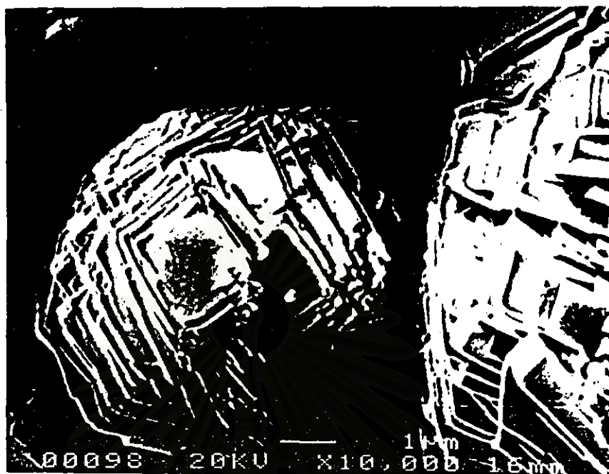
Figure 5.7 SEM photograph (x 10000) of prepared ZSM-5
