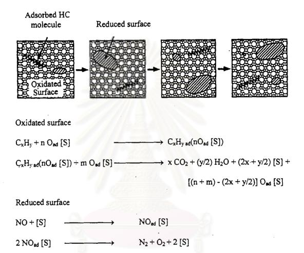
Figure 3.1 Conceptional illustration of the Microscopic Sequential Reaction mechanism for deNO<sub>x</sub> reaction under the oxygen excess condition [64]
