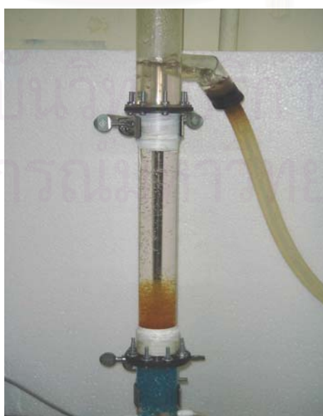
Figure 5.4 Photo of lab scale fluidized bed reactor
