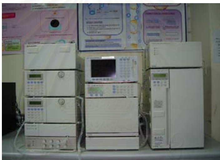
Figure 5.10 The picture of HPLC (Shimadzu column class VP)
