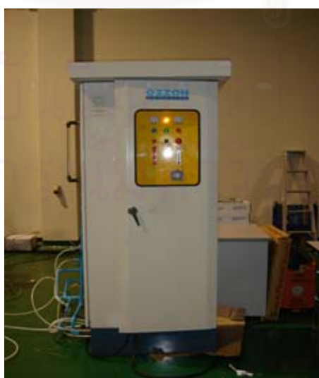
Figure 5.9 Ozone generator model OZ-7540 of Asia-Tech Engineering Co., Ltd
