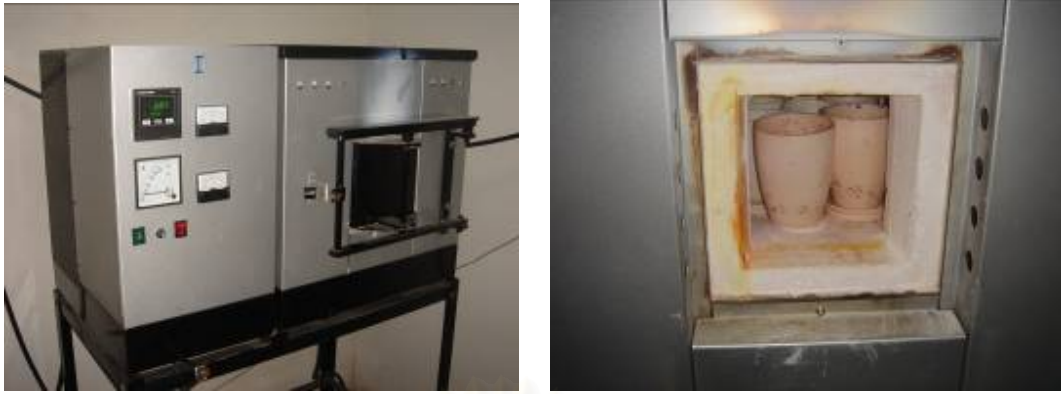
Figure 3.5 Electric furnaces in the ruby heat-treatment room of Factory A.
