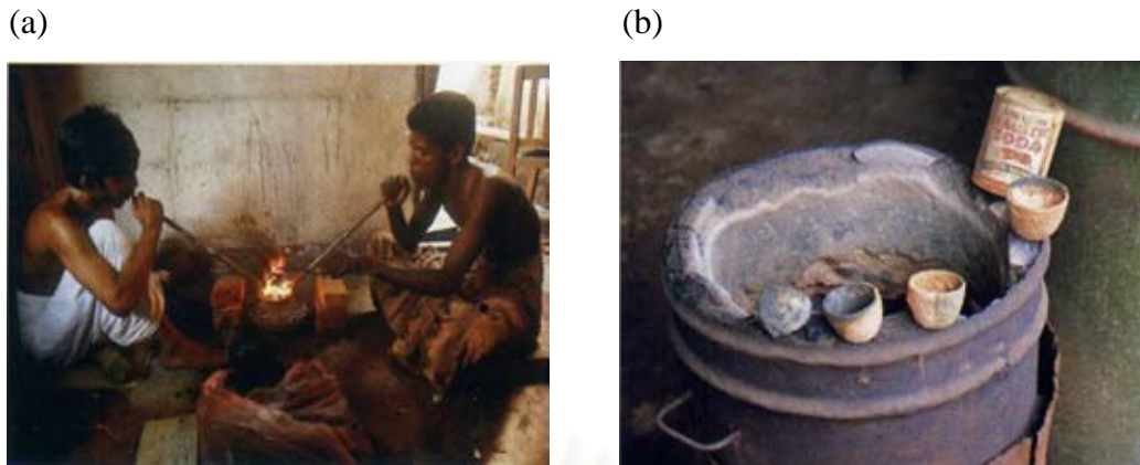
Figure 2.2 (a) The centuries old technique of blow-pipe heat treatment of ruby in Sri Lanka (b) Primitive charcoal oven at Chathaburi town, Thailand (from Hughes, 1997).
