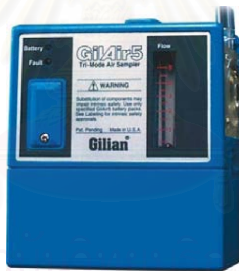
Figure 3.2 GilAir-5 constant flow air sampling pump used during this research project (from Sensidyne Inc., 2001).
