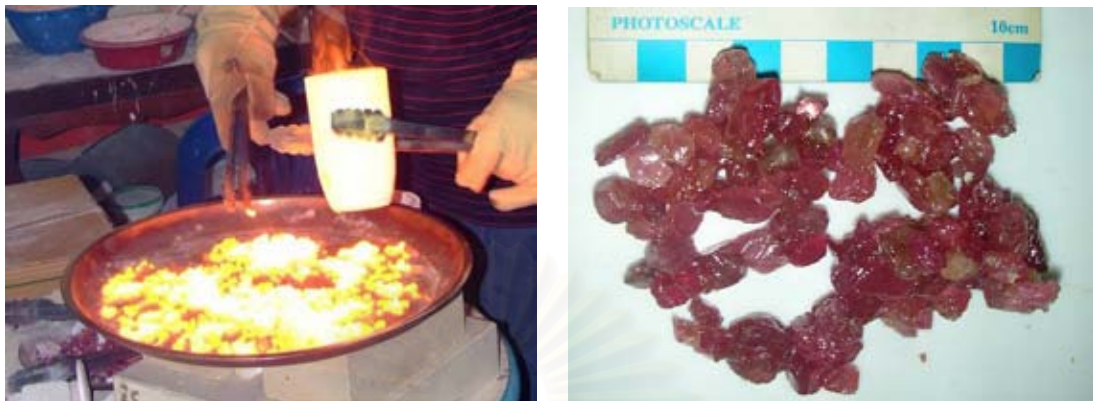
Figure 2.10 (a) Removal of the ruby from the crucible (b) Glued ruby after lead-glass filled heat treatment.
