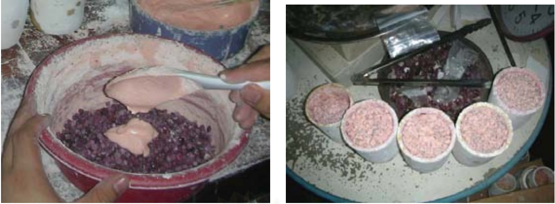
Figure 2.6 (a) Ruby soaked with lead-glass additives (b) Loading ruby mixed with lead-glass additives into crucibles.
