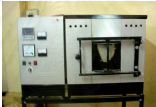
Figure 2.7 Electric furnace used in Chathaburi province, Thailand.
