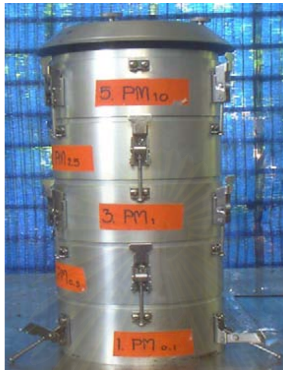
Figure 3.1 Different sizes of PUF and the size-fractionated Cascade Impactor
