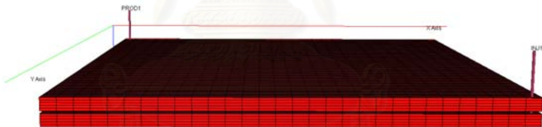
Figure 5-2: 3-dimension reservoir model of 5 vertical sub-layers per layer
