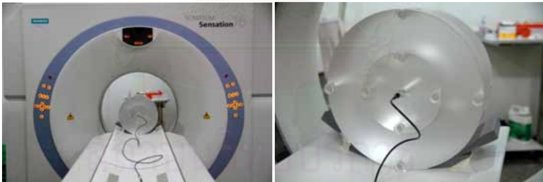
Figure 3.14 The experimental set up for the verification of CTDI_{vol} by using the 32 cm diameter PMMA phantom and the pencil ionization chamber connected with the electrometer.
