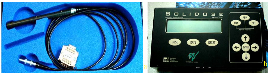
Figure 3.4 The Pencil ionization chamber (a.) and electrometer (b.) are commonly connected and inserted in a cylindrical phantom for the measurement of CT dose index.
