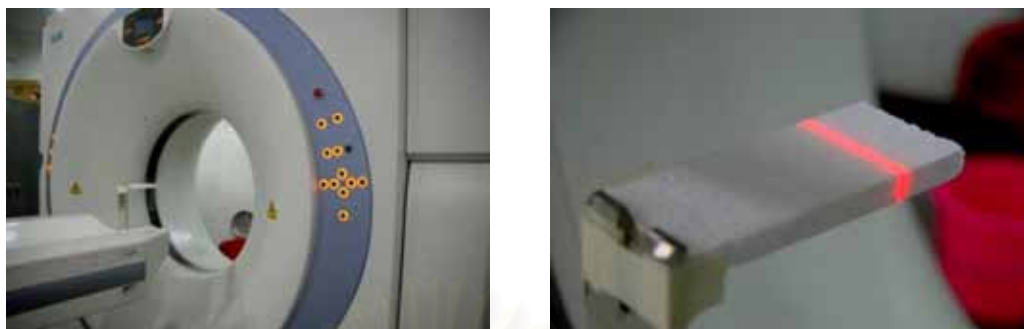
Figure 3.8 The experimental setup for evaluation of spatial resolution; (a) the micro bead of 0.38 mm in diameter was placed at 20 mm above the center of CT gantry, (b) the micro bead was fixed inside a foam support.
