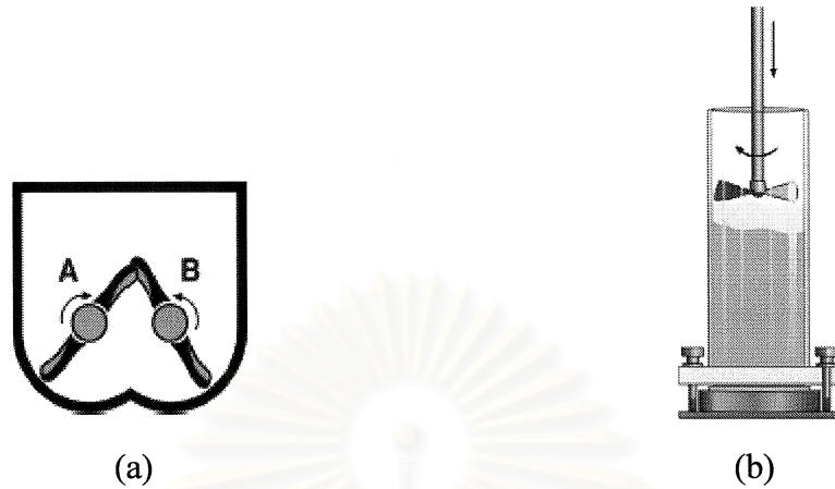
Figure 7. Instrument of torque method: (a). Mixer torque rheometer and (b) Powder rheometer (Lukkonen, 2001)
