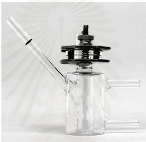
Figure 10 A side view of a joint adapter-jacketed modified Franz diffusion cell (adapted from Franz, 1975).
