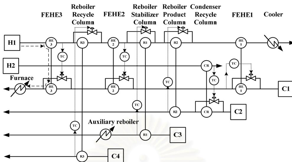
**Figure 6.63** the Heat Pathway of Control Structure with Outlet Cold Temperature Control at FEHE1 for Changing in the Heat Load Disturbance of Cold Stream by Increasing Inlet Temperature of Reactor Product Stream
