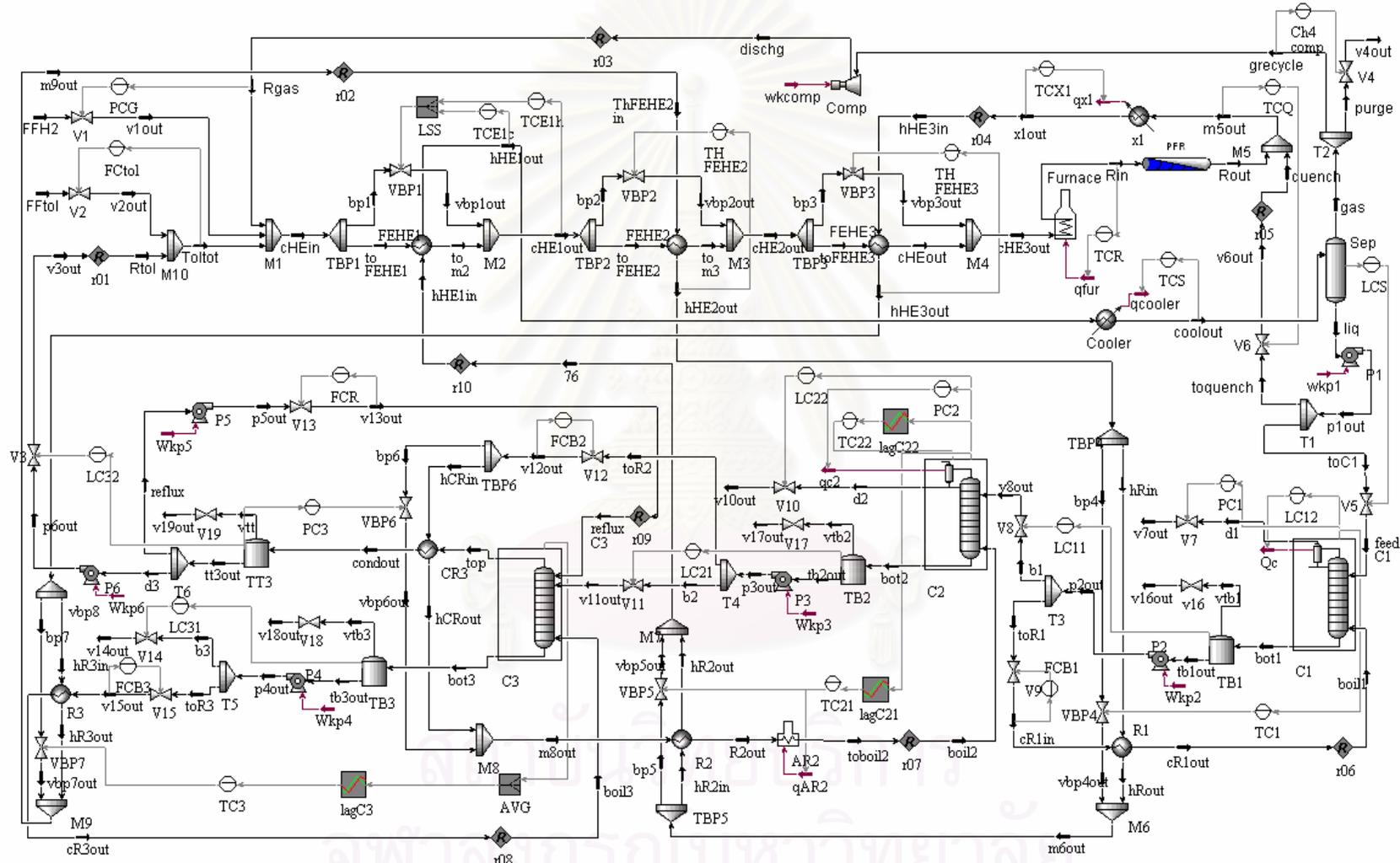
Figure 6.12 Control Structure 3 (CS3) for HDA Process Alternative 6 with Four Auxiliary Utility Units
