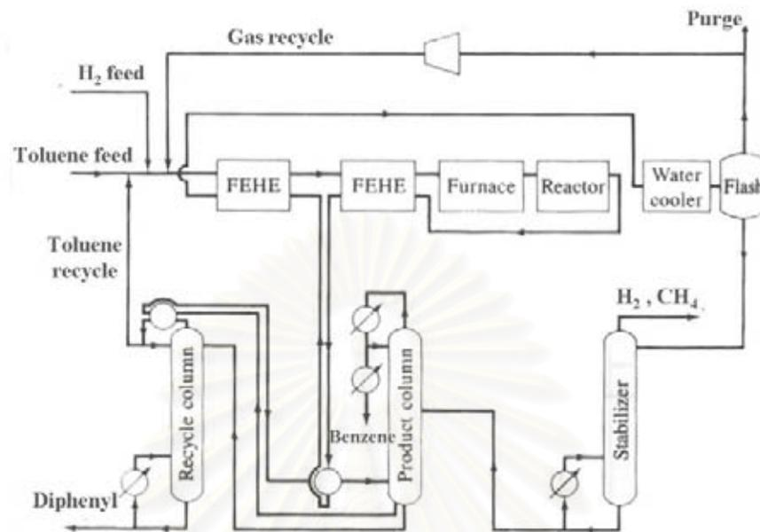
Figure 4.5 HDA process –alternative 4
