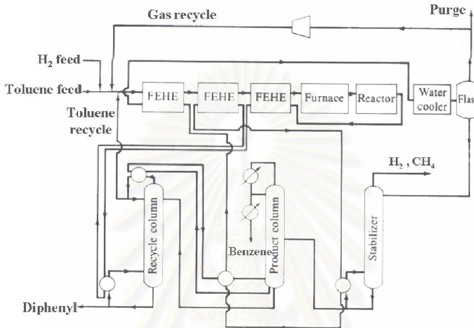
Figure 4.7 HDA process –alternative 6
