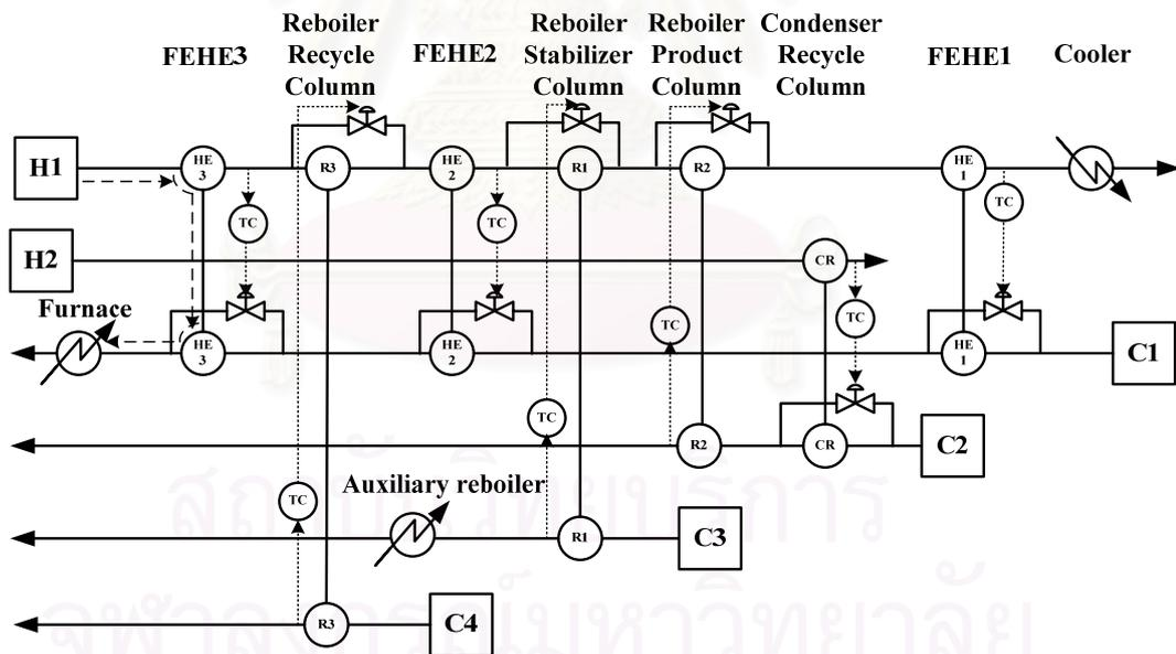
**Figure 6.59** The Heat Pathway of Control Structure with outlet hot temperature control at FEHE1 for Changing in the Heat Load Disturbance of Cold Stream by Decreasing Inlet Temperature of Reactor Product Stream
