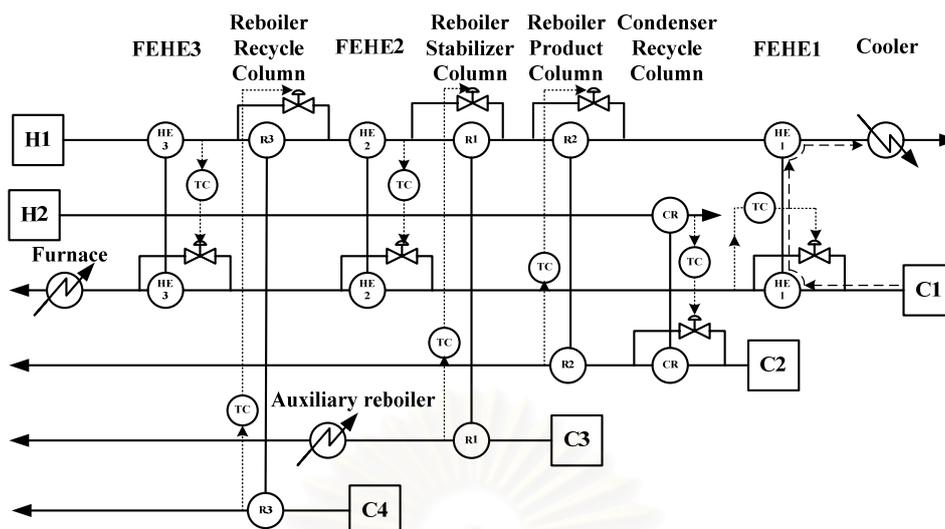
**Figure 6.54** the Heat Pathway of Control Structure with Outlet Cold Temperature Control at FEHE1 for Changing in the Heat Load Disturbance of Cold Stream by Decreasing Inlet Temperature of Reactor Feed Stream
