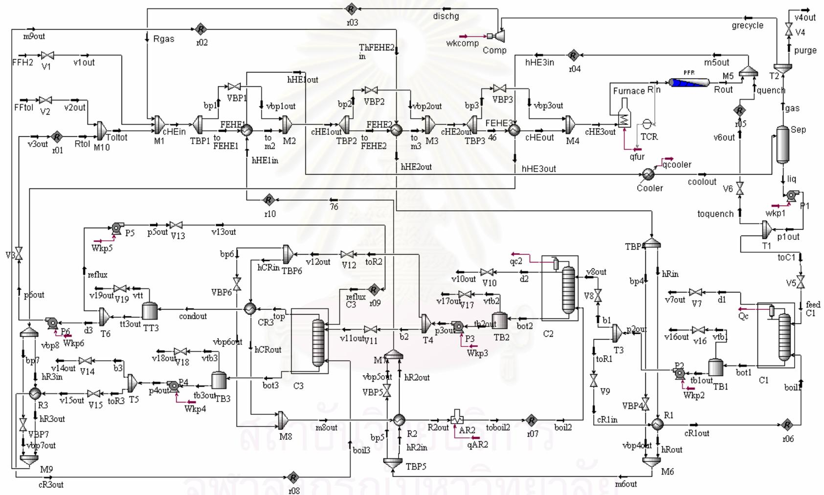
**Figure 5.24** Hysy Flowsheet of the Steady State Modeling of HDA Process Alternative 6 with Minimum Auxiliary Utility Unit
