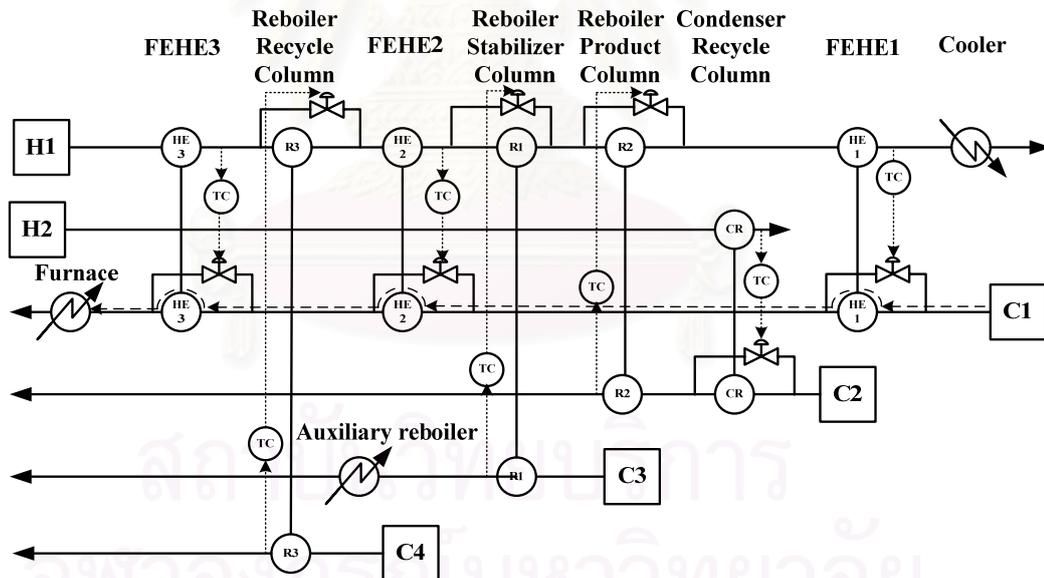
**Figure 6.53** the Heat Pathway of Control Structure with Outlet Hot Temperature control at FEHE1 for Changing in the Heat Load Disturbance of Cold Stream by Decreasing Inlet Temperature of Reactor Feed Stream
