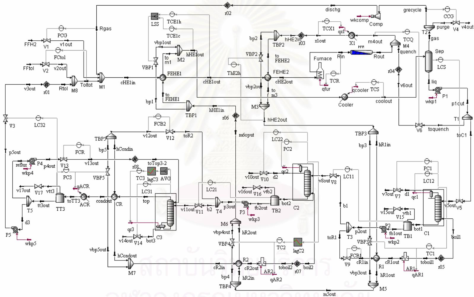
Figure 6.2 Control Structure 2 (CS2) for HDA Process Alternative 5 with three Auxiliary Utility Units
