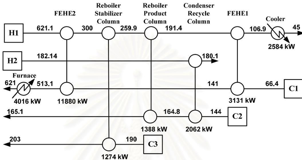
**Figure 5.8** the Heat Exchanger Network of HDA Process Alternative 5 at Normal Operating Condition
