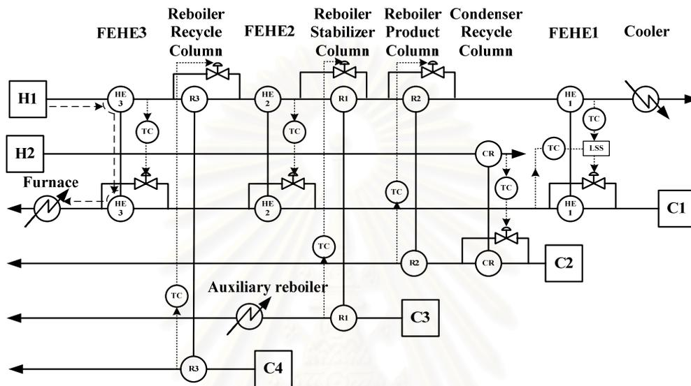
**Figure 6.61** the Heat Pathway of Control Structure with LSS at FEHE1 for Changing in the Heat Load Disturbance of Cold Stream by Increasing Inlet Temperature of Reactor Product Stream
