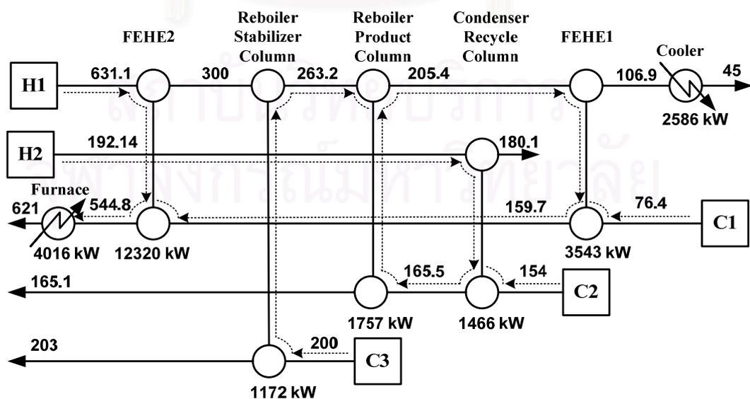
**Figure 5.10** the Heat Exchanger Network of HDA Process Alternative 5 at Maximum Cooling Condition
