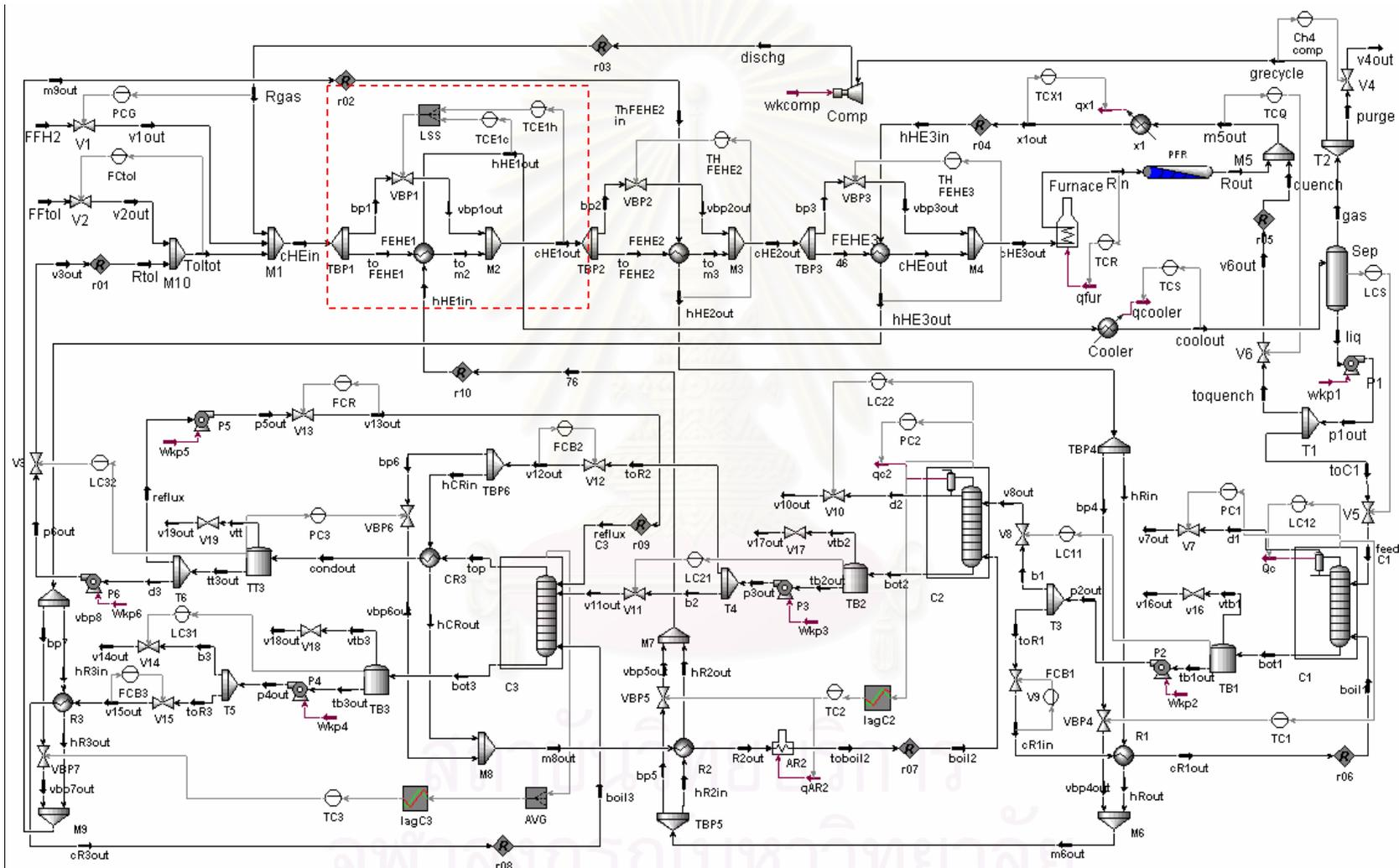
Figure 6.49 Control Structure with Low Selective Switch (LSS) of Selective Controller at FEHE1
