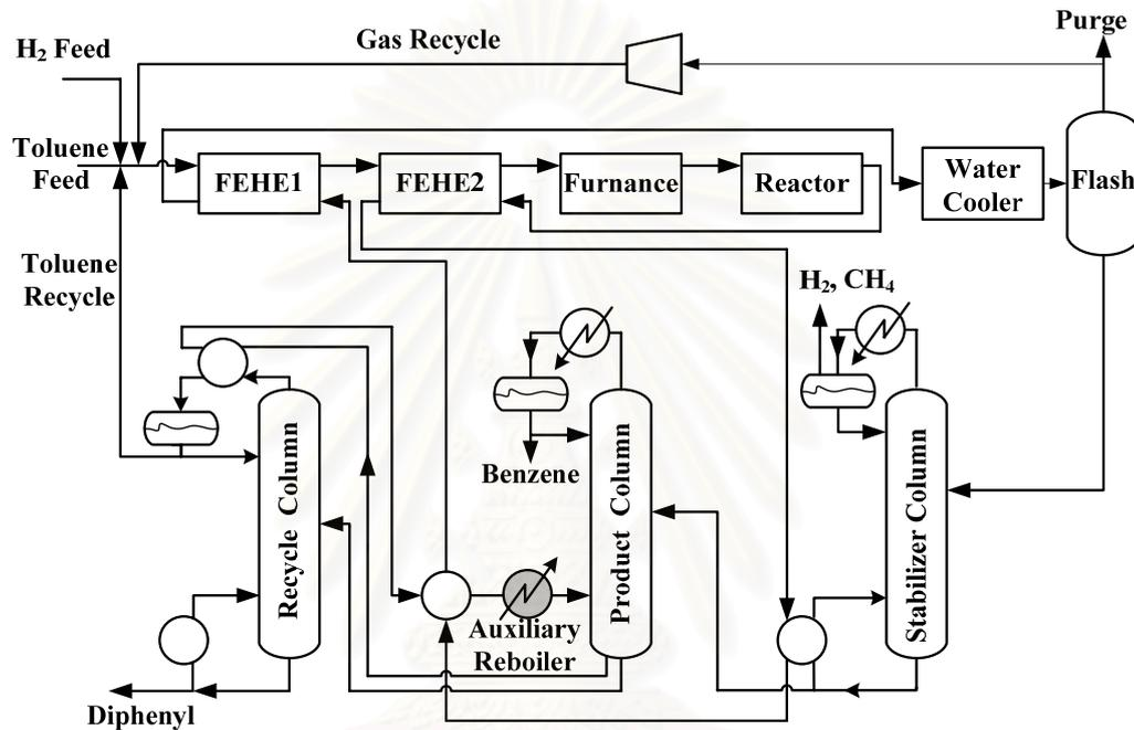
**Figure 5.11** the HDA Process Alternative 5 with Minimum Auxiliary Utility Unit
