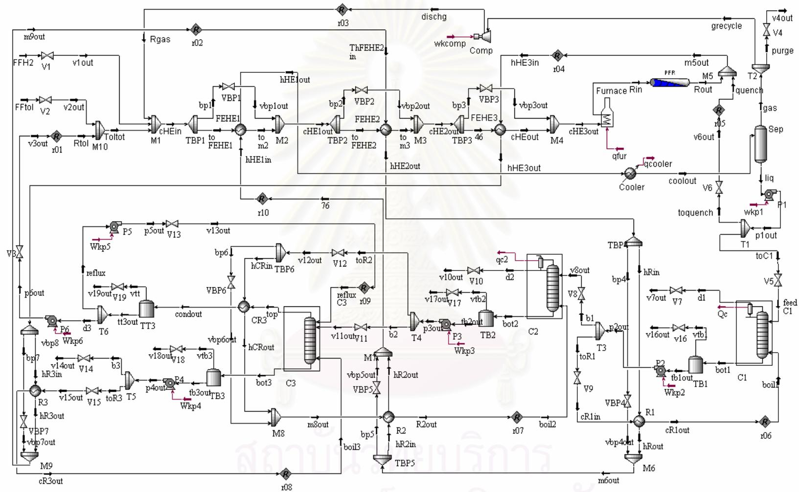
Figure 4.9 Hysy Flowsheet of the Steady State Modeling of HDA Process Alternative 6
