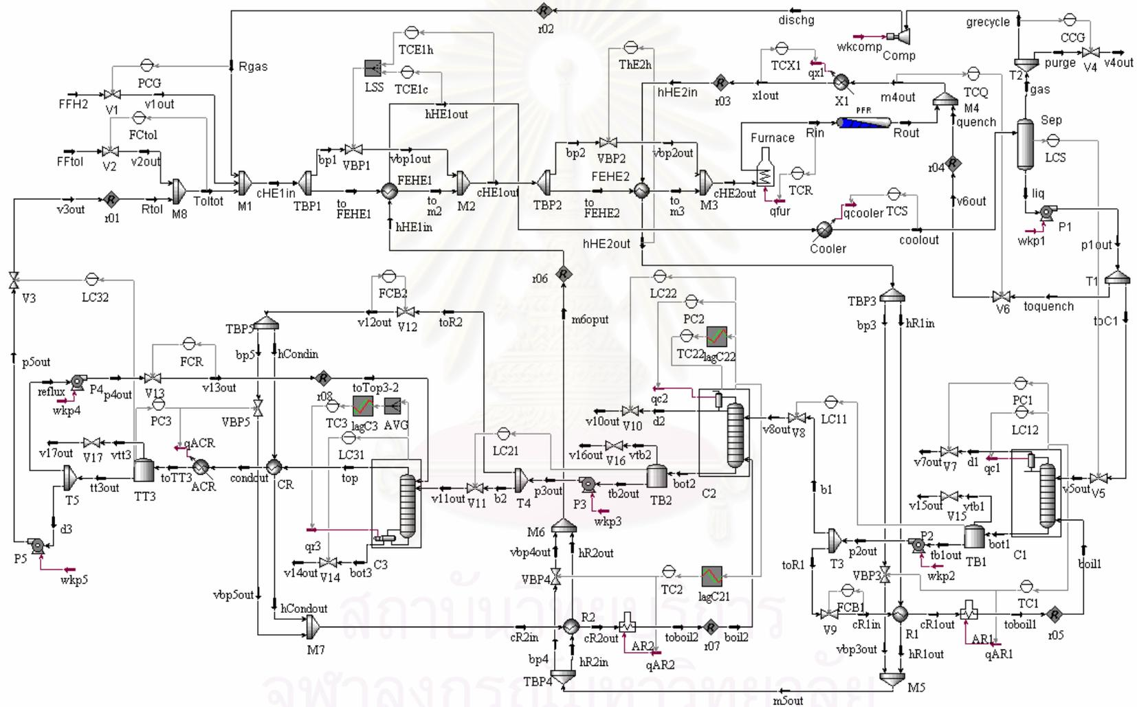
Figure 6.3 Control Structure 3 (CS3) for HDA Process Alternative 5 with three Auxiliary Utility Units
