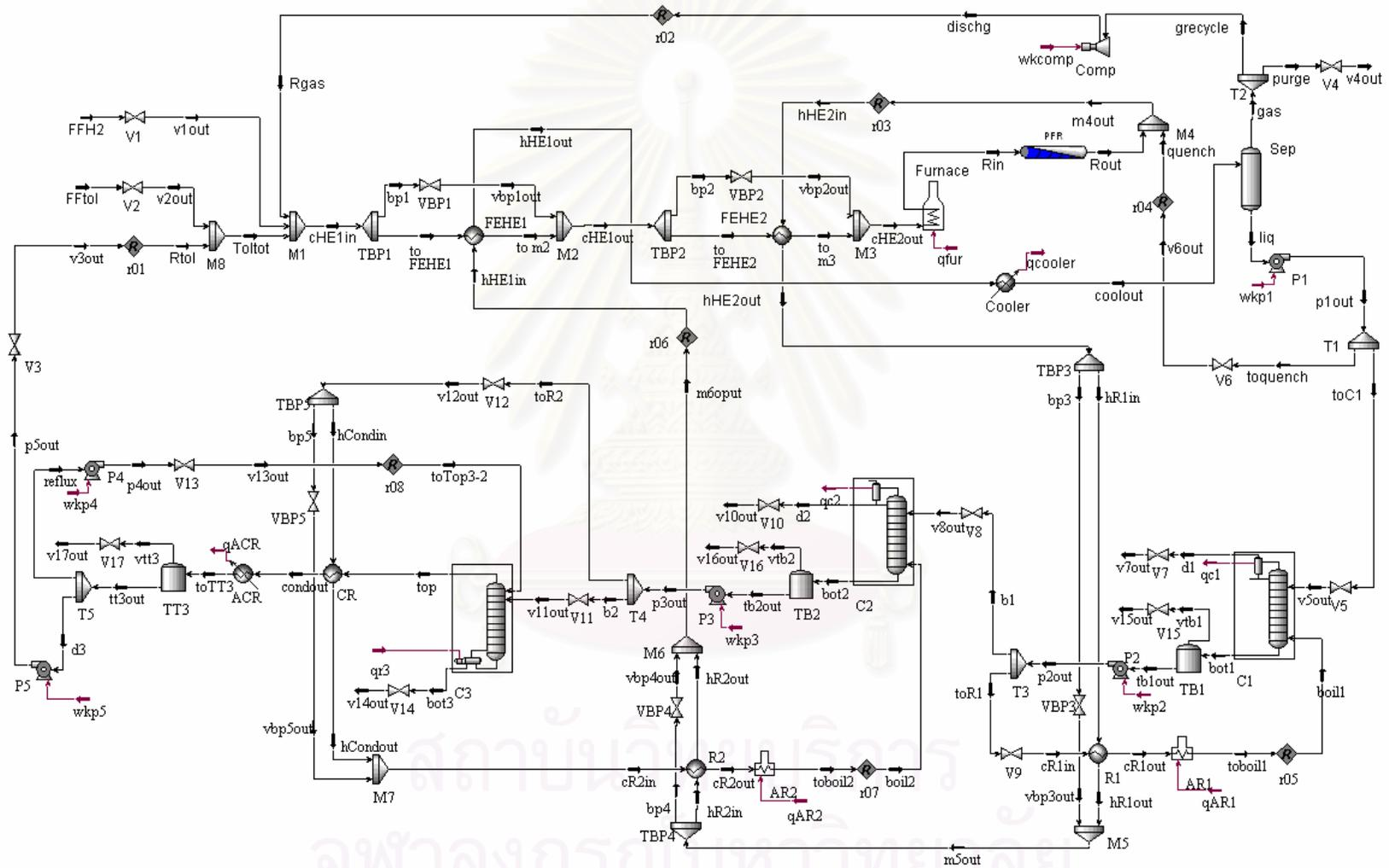
**Figure 5.21** Hysy Flowsheet of the Steady State Modeling of HDA Process Alternative 5 with three Auxiliary Utility Unit
