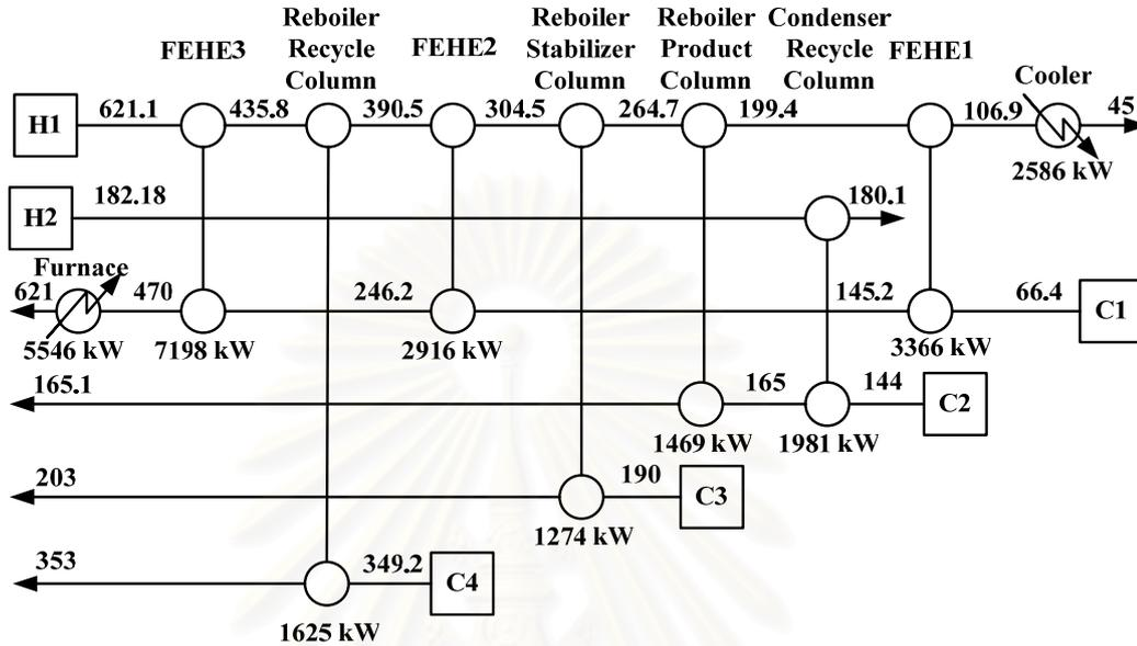
**Figure 5.15** the Heat Exchanger Network of HDA Process Alternative 6 at Normal Operating Condition
