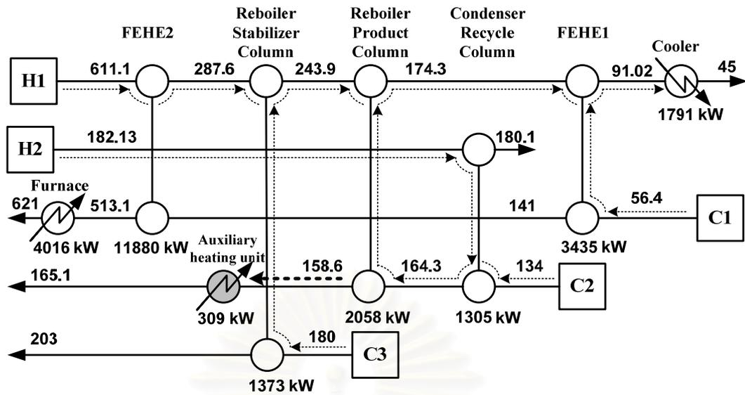
**Figure 5.9** the Heat Exchanger Network of HDA Process Alternative 5 at Minimum Heating Condition
