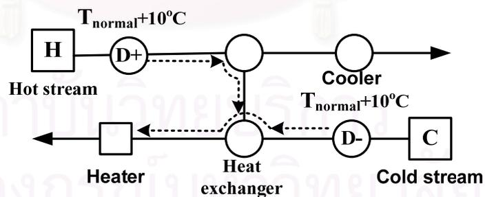
**Figure 5.4** the Appropriate Heat Pathway for the Worst Case Condition a) minimum heating condition b) maximum cooling condition
