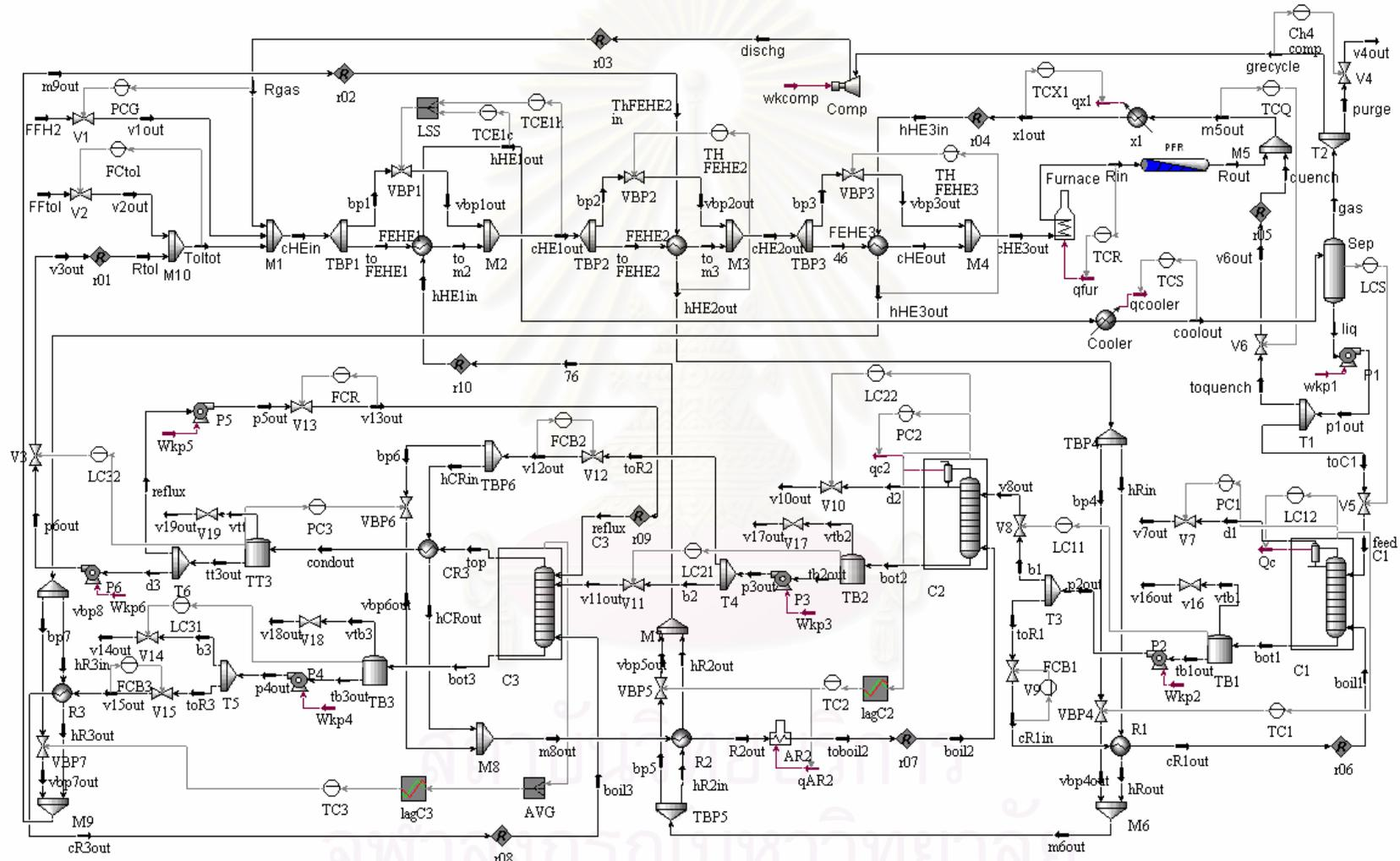
Figure 6.10 Control Structure 1 (CS1) for HDA Process Alternative 6 with Minimum Auxiliary Utility Units
