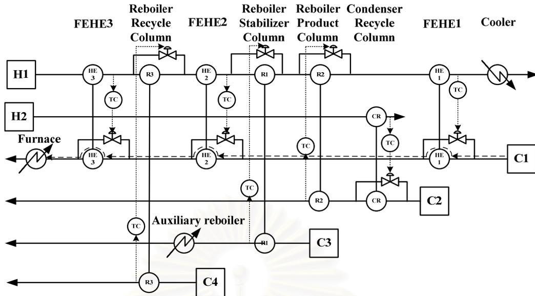
**Figure 6.56** the Heat Pathway of Control Structure with Outlet Hot Temperature control at FEHE1 for Changing in the Heat Load Disturbance of Cold Stream by Increasing Inlet Temperature of Reactor Feed Stream
