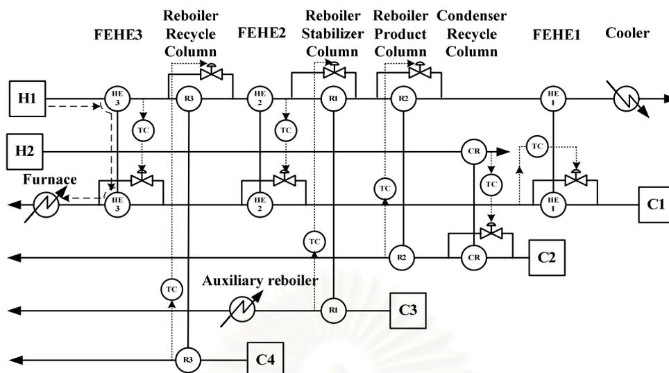
**Figure 6.60** The Heat Pathway of Control Structure with Outlet Cold Temperature Control at FEHE1 for Changing in the Heat Load Disturbance of Cold Stream by Decreasing Inlet Temperature of Reactor Product Stream
