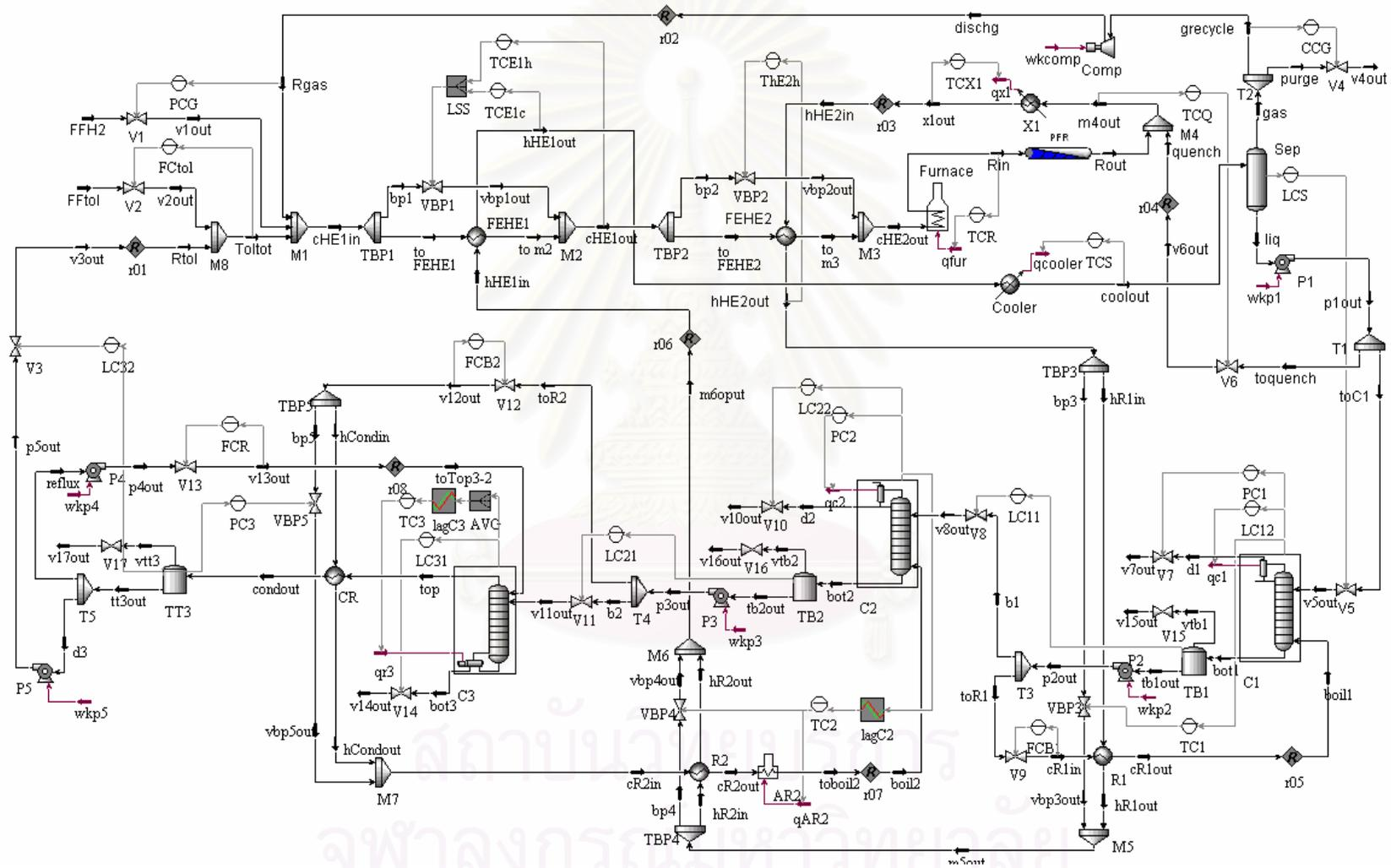
Figure 6.4 Control Structure 1 (CS1) for HDA Process Alternative 5 with Minimum Auxiliary Utility Units
