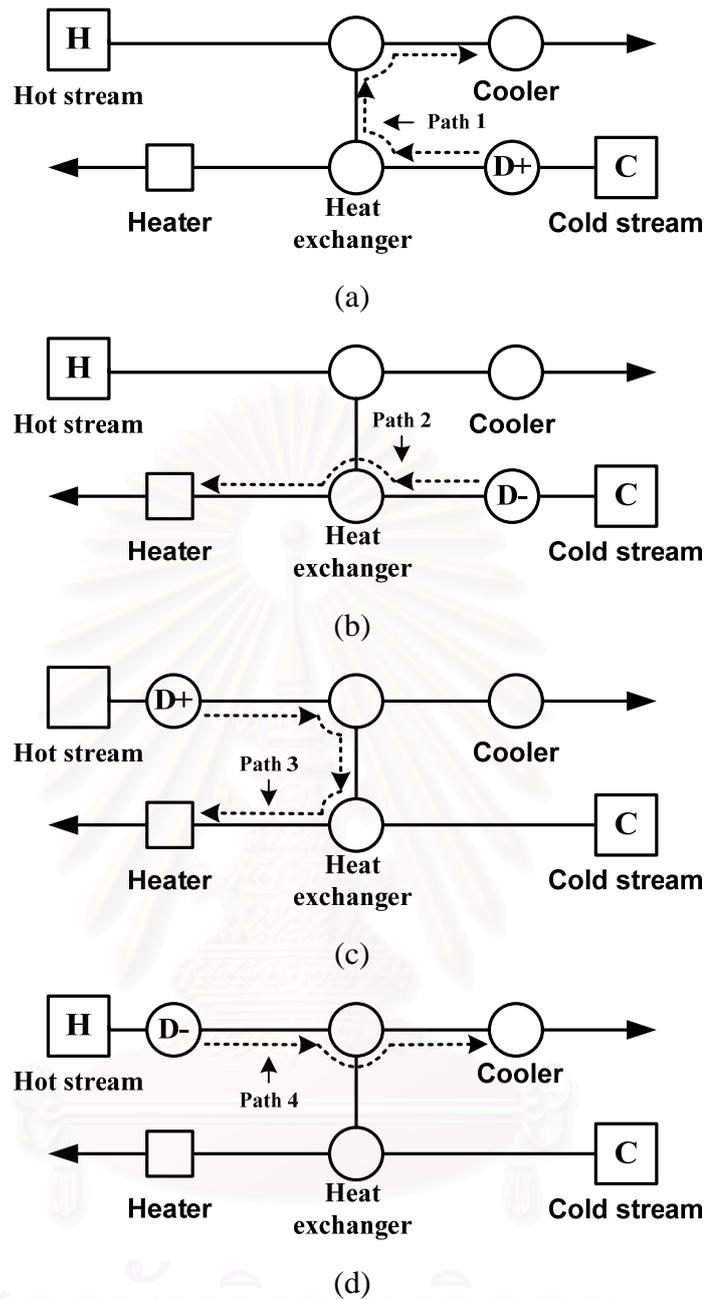
**Figure 5.3** Heat Pathways through HEN with single heat exchanger to achieve DMER, where: (a) path 1 is used to shift the positive disturbance load of the cold stream to the cooler, (b) path 2 is used to shift the negative disturbance load of the cold stream to heater, (c) path 3 is used to shift the positive disturbance load of the hot stream to heater, and (d) path 4 is used to shift the negative disturbance load of hot stream to the cooler.
