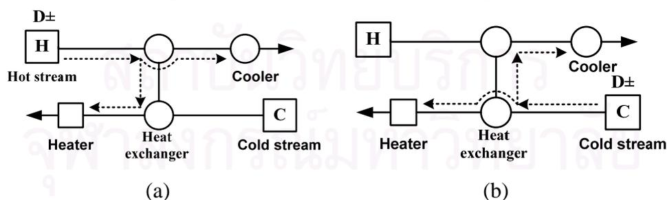
**Figure 5.2** the Disturbance Load is Propagated to Heater and Cooler (a) positive and negative disturbance load in hot stream cases (b) positive and negative disturbance load in cold stream cases
