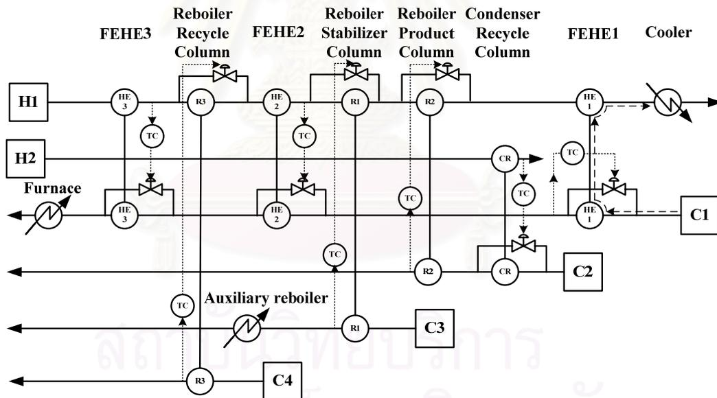
**Figure 6.57** the Heat Pathway of Control Structure with Outlet Cold Temperature Control at FEHE1 for Changing in the Heat Load Disturbance of Cold Stream by Increasing Inlet Temperature of Reactor Feed Stream
