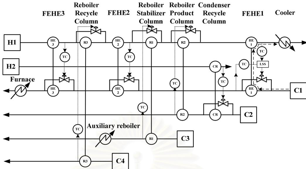
**Figure 6.52** the Heat Pathway of Control Structure with LSS at FEHE1 for Changing in the Heat Load Disturbance of Cold Stream by Decreasing Inlet Temperature of Reactor Feed Stream
