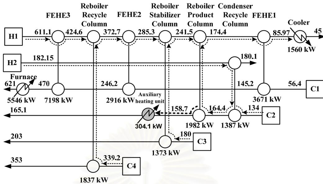
**Figure 5.16** the Heat Exchanger Network of HDA Process Alternative 6 at Minimum Heating Condition
