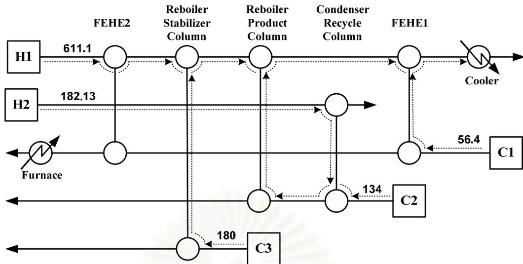
**Figure 5.6** Design Heat Pathway at Minimum Heating Condition for Heat Exchanger Network HDA Alternative 5
