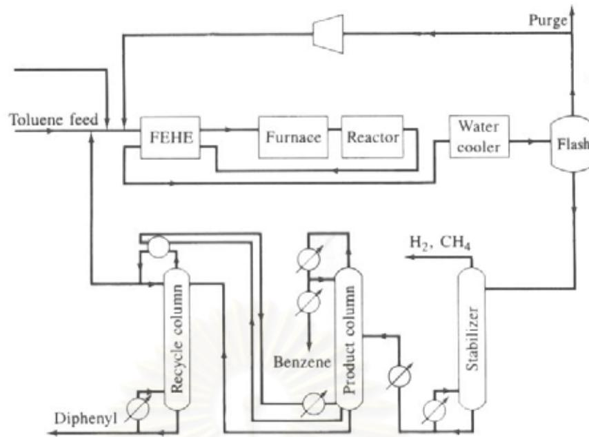
Figure 4.3 HDA process –alternative 2
