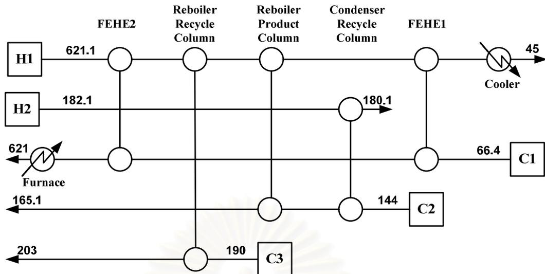
**Figure 5.5** Heat Exchanger Network of HDA Process Alternative 5
