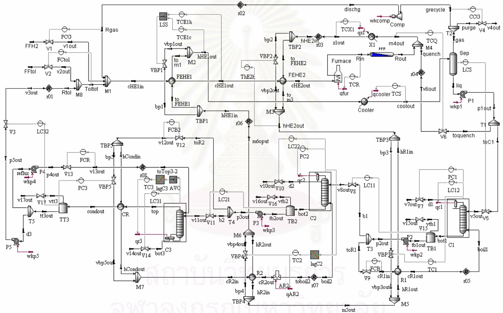
Figure 6.5 Control Structure 2 (CS2) for HDA Process Alternative 5 with Minimum Auxiliary Utility Units
