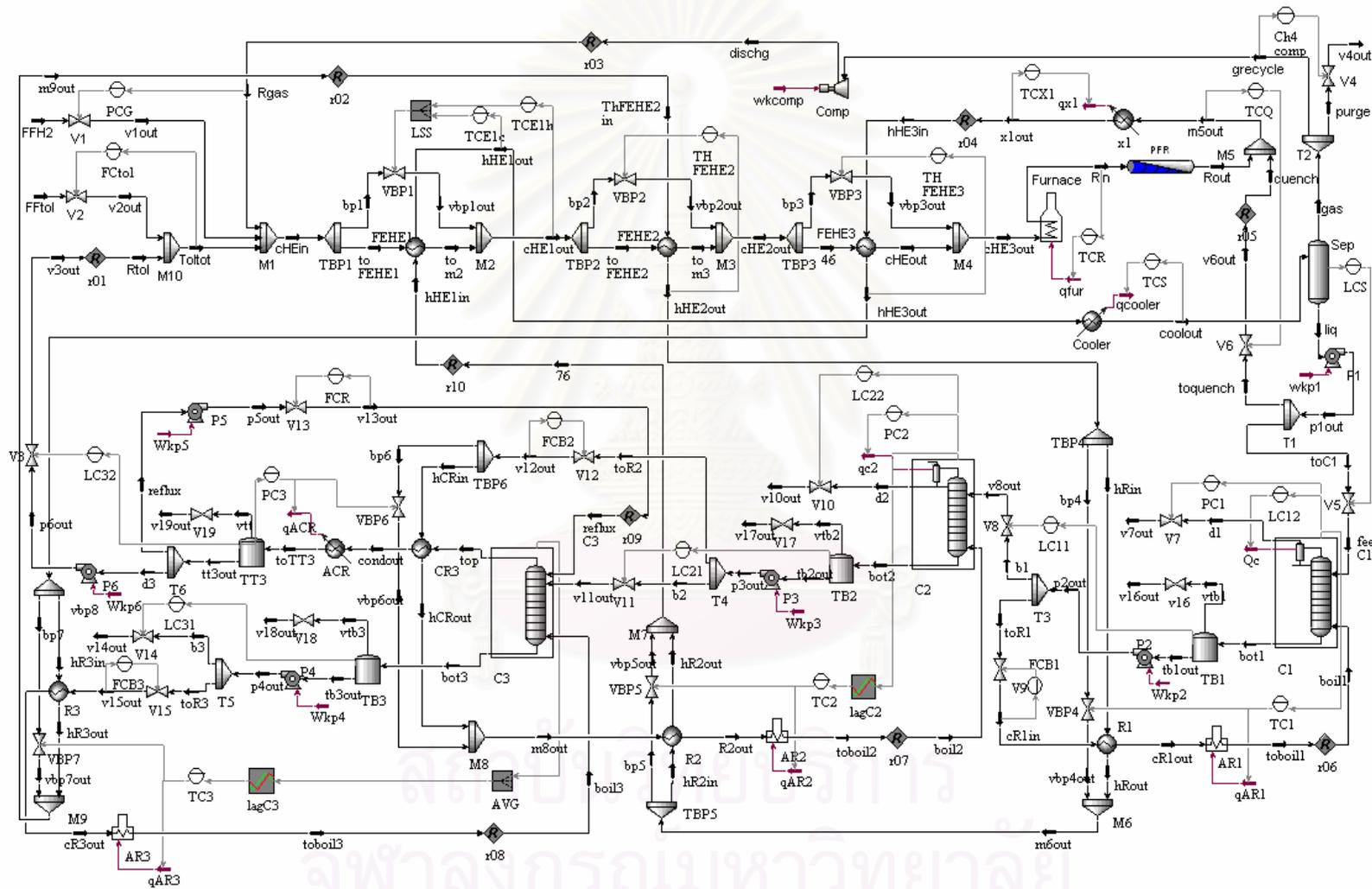
**Figure 6.7** Control Structure 1 (CS1) for HDA Process Alternative 6 with four Auxiliary Utility Units
