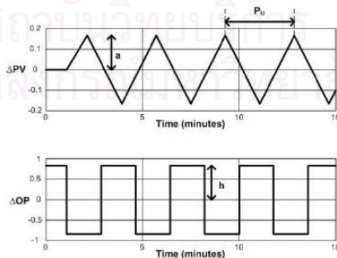
**Figure C.1** Input and Output from Relay-Feedback Test
