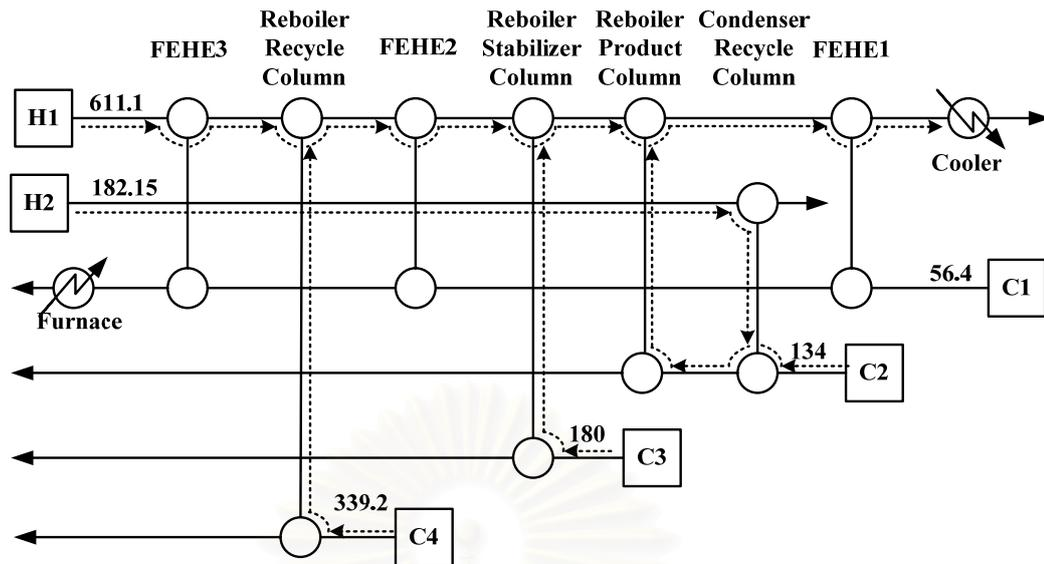
**Figure 5.13** Design Heat Pathway at Minimum Heating Condition for Heat Exchanger Network HDA Alternative 6
