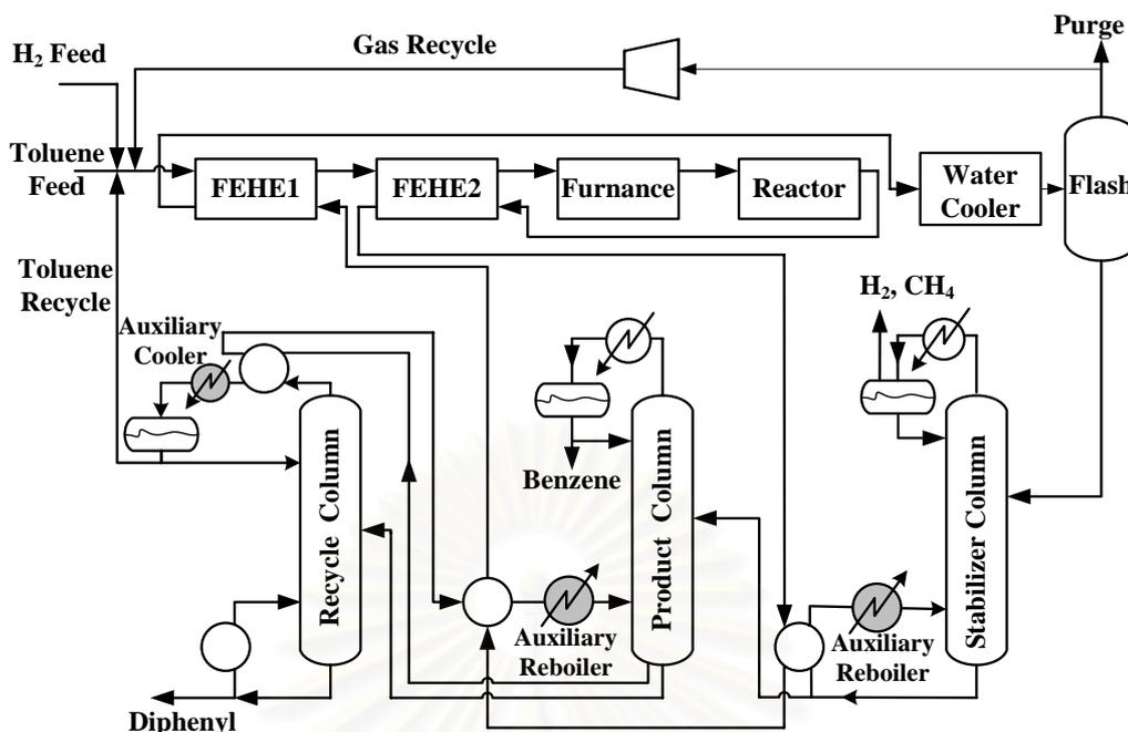
**Figure 5.19** HDA Process Alternative 5 with two Auxiliary Reboilers and one Auxiliary Cooler
