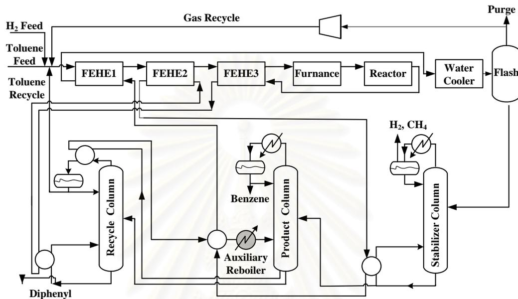
**Figure 5.18** the HDA Process Alternative 6 with Minimum Auxiliary Utility Unit
