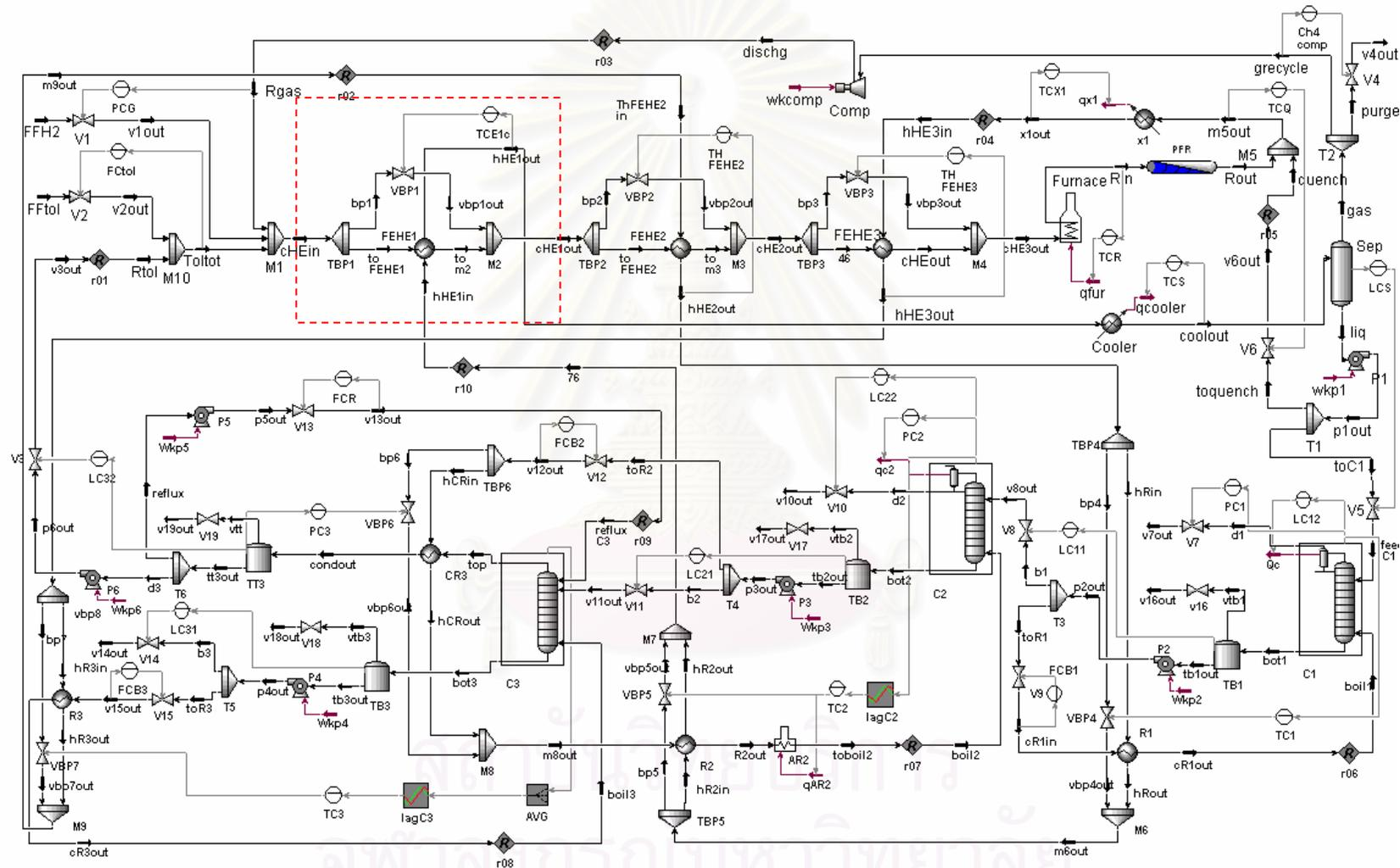
Figure 6.50 Control Structure with outlet hot temperature control at FEHE1
