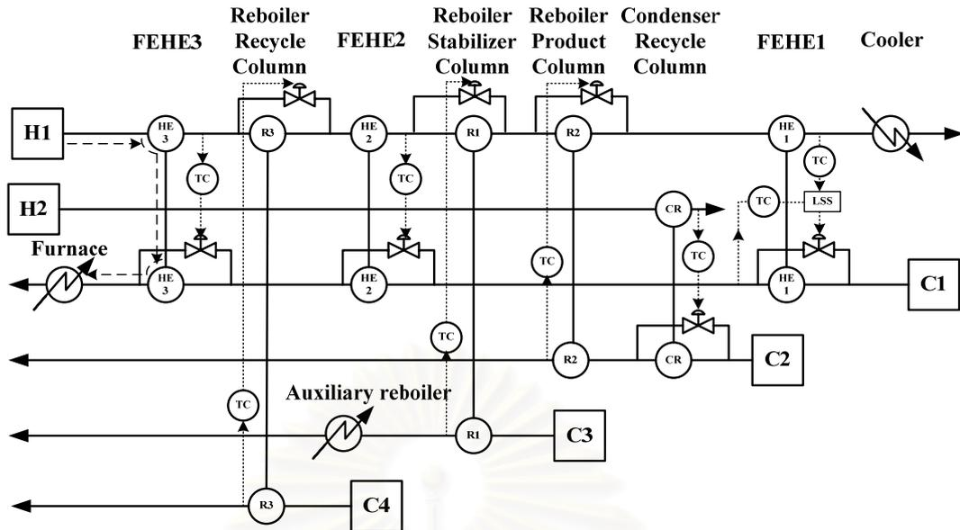
**Figure 6.58** the Heat Pathway of Control Structure with LSS at FEHE1 for Changing in the Heat Load Disturbance of Cold Stream by Decreasing Inlet Temperature of Reactor Product Stream
