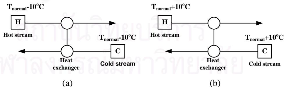
**Figure 5.1** Worst Case Condition (a) Minimum heating (b) Maximum cooling condition
