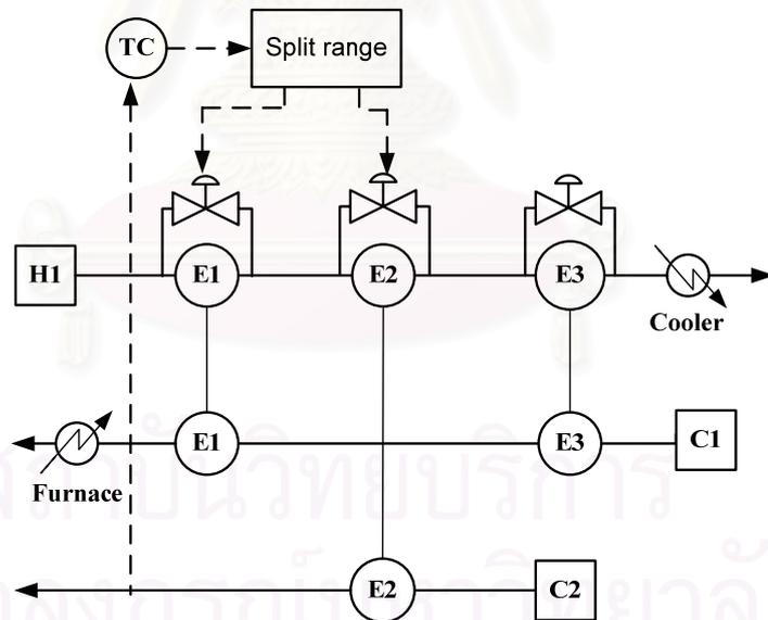
**Figure 7.1** The example modifying control structure for the process with out auxiliary utility unit
