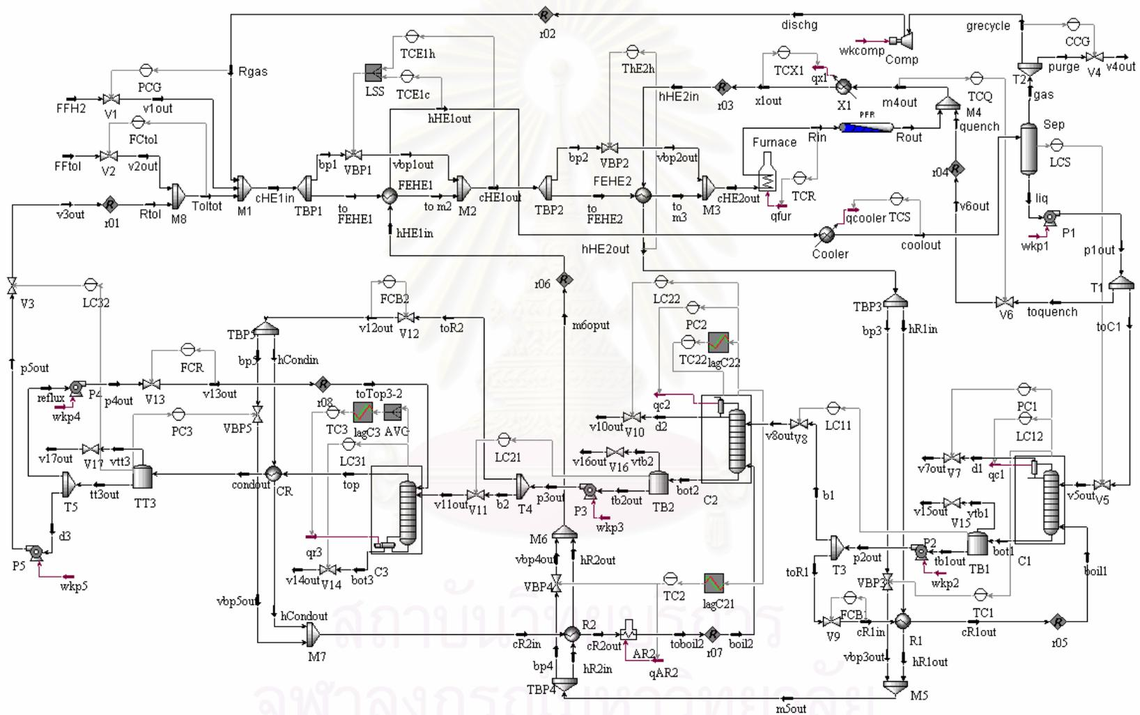
Figure 6.6 Control Structure 3 (CS3) for HDA Process Alternative 5 with Minimum Auxiliary Utility Units
