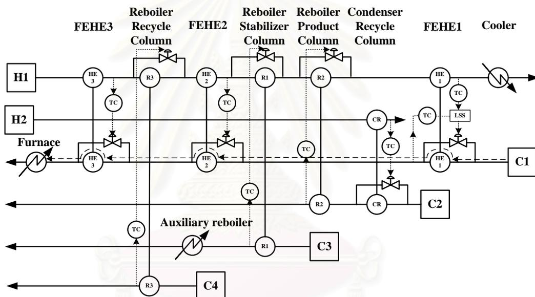
**Figure 6.55** the Heat Pathway of Control Structure with LSS at FEHE1 for Changing in the Heat Load Disturbance of Cold Stream by Increasing Inlet Temperature of Reactor Feed Stream
