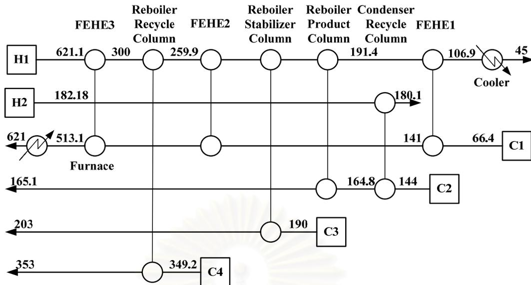
**Figure 5.12** Heat Exchanger Network of HDA Process Alternative 6
