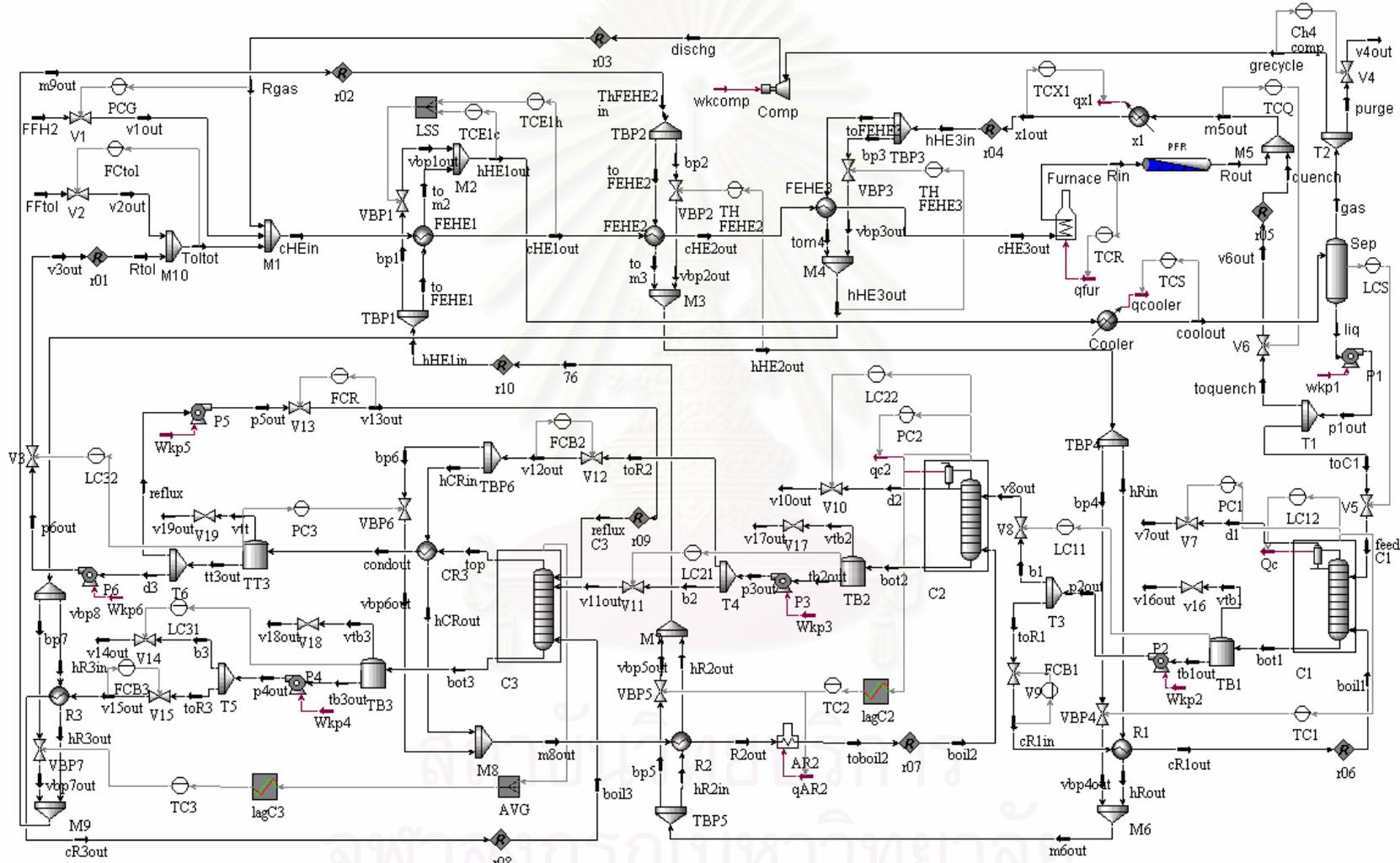
Figure 6.11 Control Structure 2 (CS2) for HDA Process Alternative 6 with Minimum Auxiliary Utility Units
