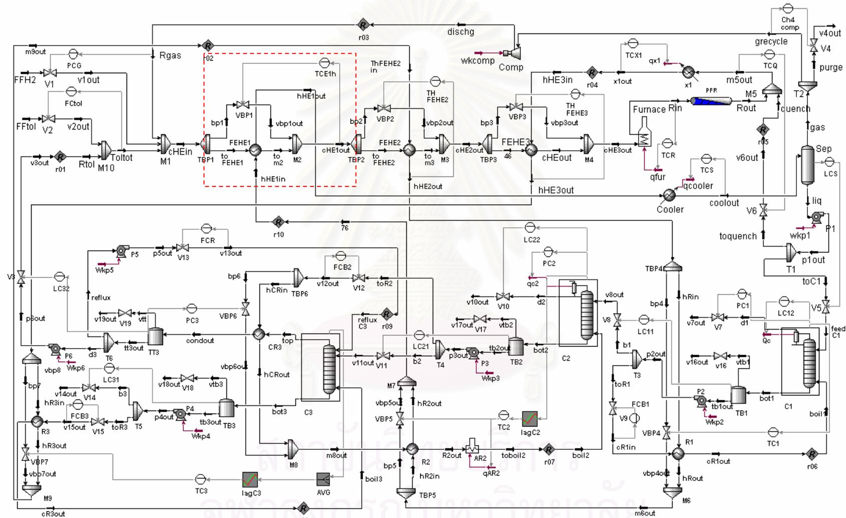
Figure 6.51 Control Structure with outlet cold temperature control at FEHE1
