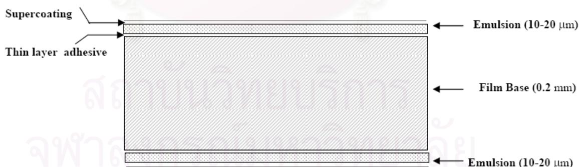
**Figure 2.16** Cross-section of a double emulsion X-ray film.
