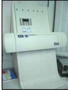
**Figure 3.5** Vidar film digitizer (VXR-16 pro dosimetry, Vidar systems Corp., Herndon, VA)
