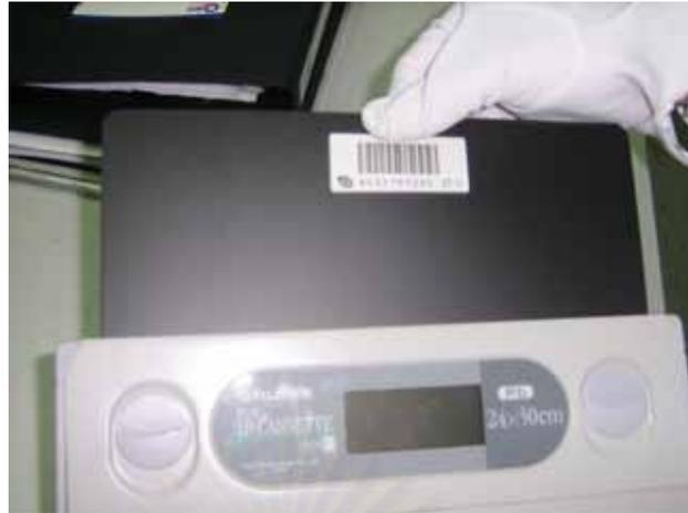
**Figure 3.1** Fuji Computed radiography imaging plate.
