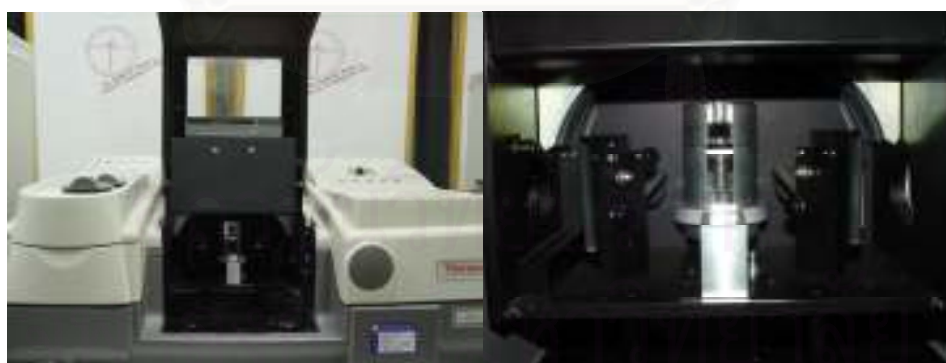
Figure 3.7 Single-reflection attenuated total reflection accessory (The Seagull TM , Harrick Scientific, USA) with a hemispherical Ge IRE at the incident angle of 30°.
