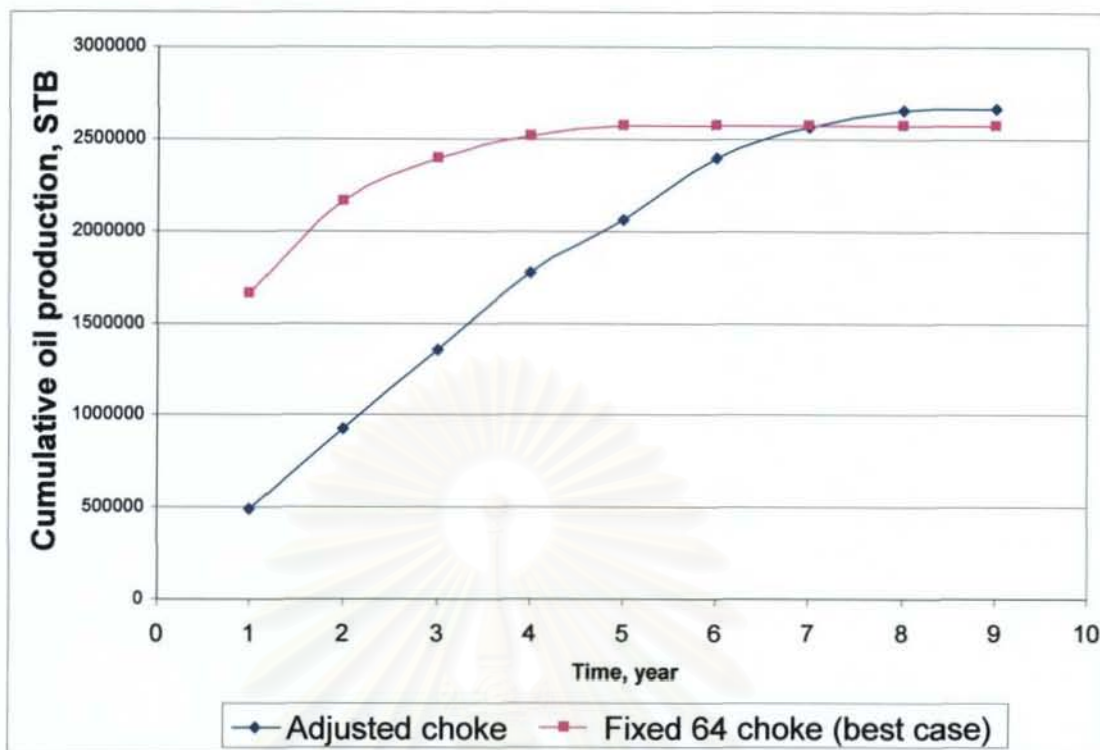
Figure 3.9: Comparison of cumulative oil productions between fixed 64 choke and 32-64 adjusted choke.
