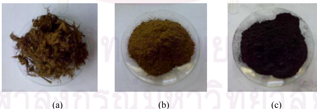
Figure 4.1 (a) Eucalyptus bark before crushed and sieved (b) Eucalyptus bark after crushed and sieved (c) activated carbon from Eucalyptus bark
