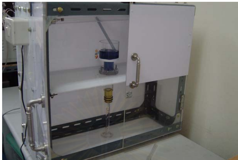
Figure 3.10. The apparatus for preventing loss of titanium dioxide by immobilization as cake layer
