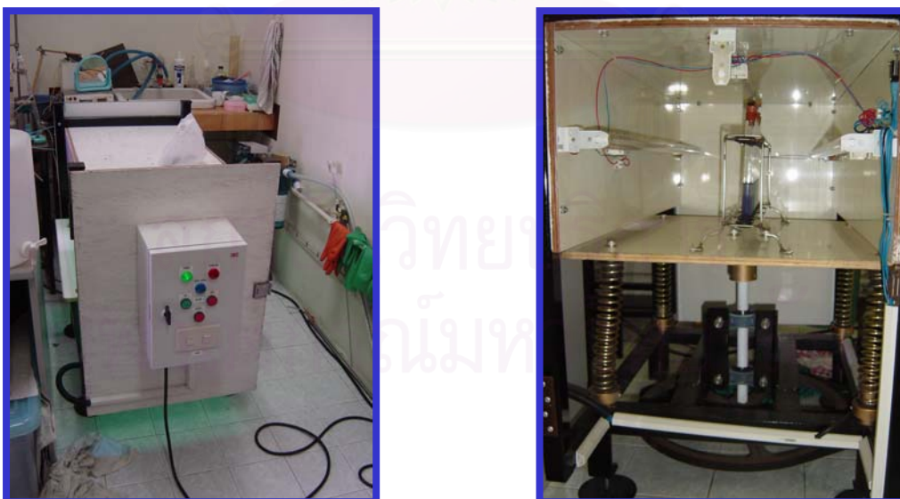
Figure 3.2. Outside (left) and inside (right) of shaker
