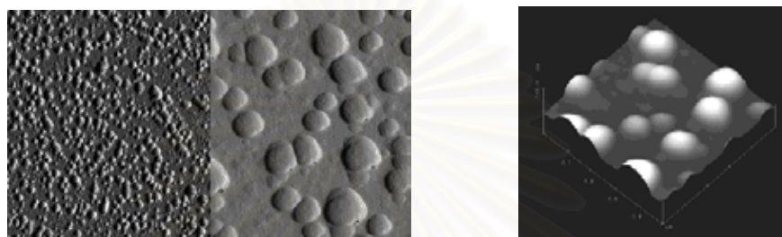
Figure 1.4 Atomic force micrograph of poly[(vinyl-3-(diethylamino)-propylcarbamate- co -(vinyl acetate)- co -(vinyl alcohol)]-graft-poly(L-lactic acid) nanoparticles (this figure is taken from reference 28).
