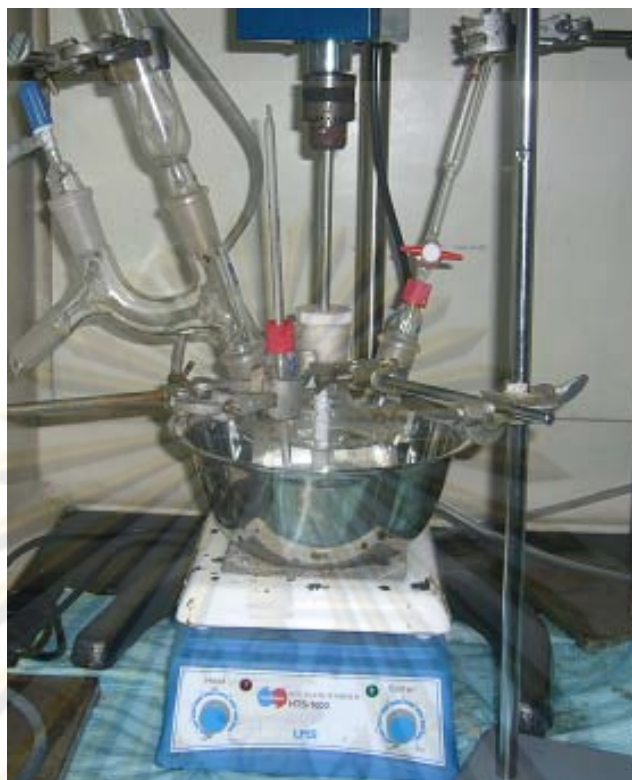
Figure 3.1 Apparatus for emulsion graft copolymerization.
