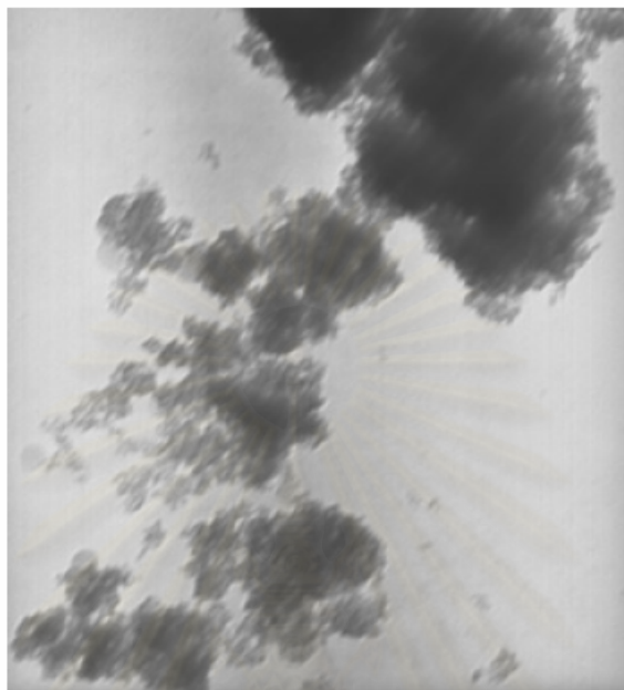
Figure 2. The TEM image of titania nanoparticles that were fired at 350 °C for 2 hours.
