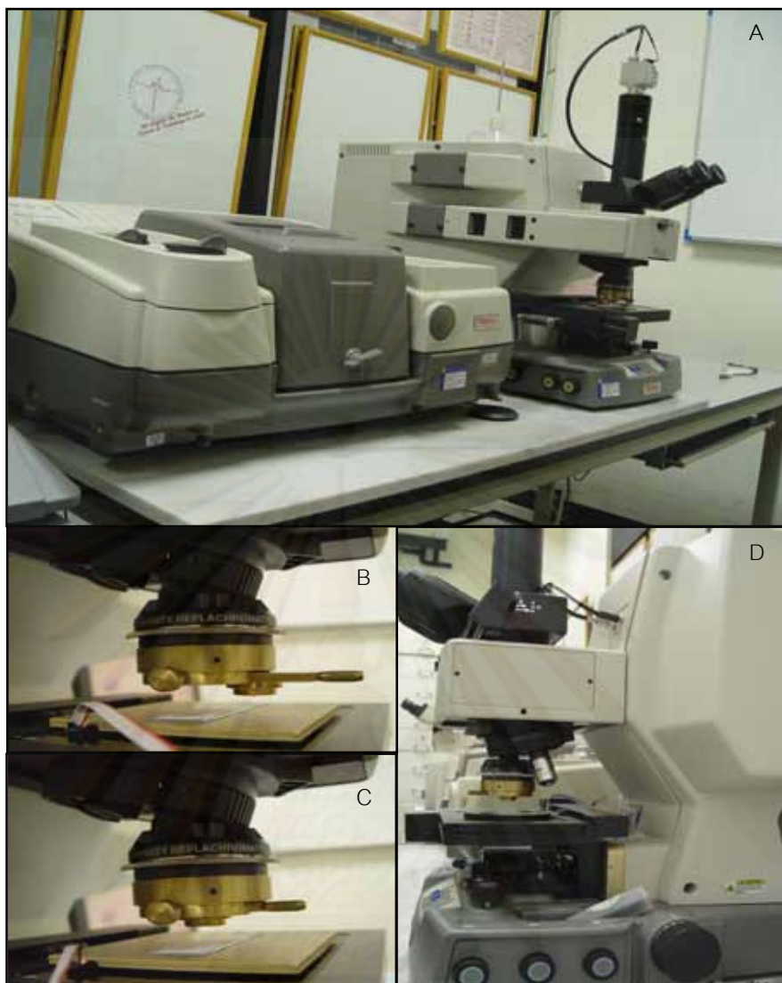
Figure 4.2. The homemade slide-on diamond \mu IRE was fixed on the 15X Schwarzschild-Cassegrain infrared objectives: (A) picture of Nicolet 6700 equipped with infrared microscope, (B) slide-on diamond \mu IRE was fixed on infrared microscope, (C) slide-on diamond \mu IRE was fixed on infrared microscope and aligned to high energy throughput, and (D) infrared microscope.
