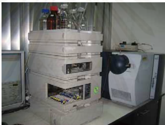
Figure 3.2 HPLC directly connected with ESI-IT mass spectrometer.
