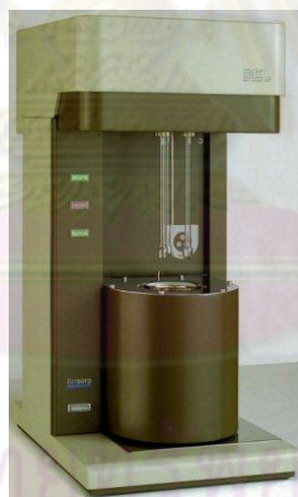
Figure 3.1 Automatic specific surface area/pore size distribution measurement (BELSORP mini, BEL Japan, Japan)
