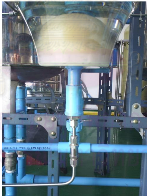
Figure 3.16 Swagelok stainless steel, check valve and air distributor
