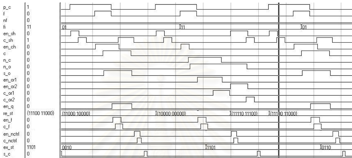
Figure 6.4: Simulation result of asynchronous dynamic pipeline control unit
