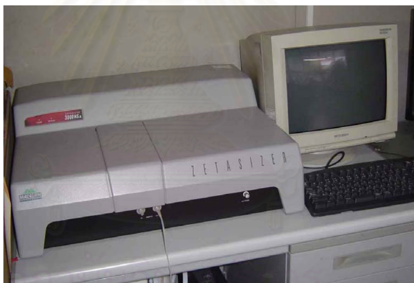
Figure 4.5 Dynamic Light Scattering (DLS) (MALVERN ZETASIZER300HSA)
