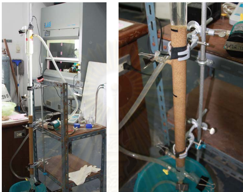
Figure A.3 Fluidized-bed Fenton experiment.
