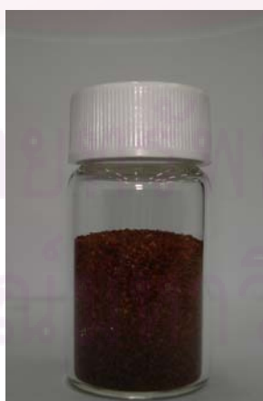
Figure A.6 Physical appearance of the iron-coated construction sand after 101-cycle crystallization.
