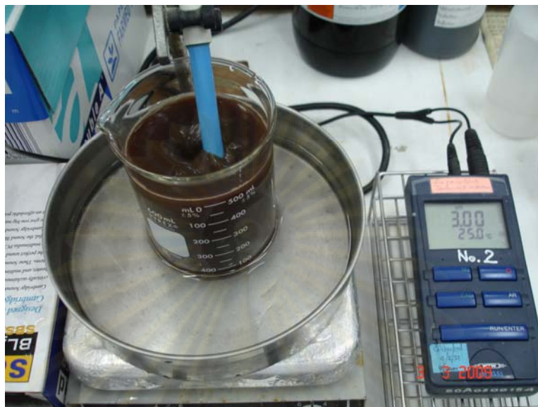
Figure A.1 Fenton experiment in the batch mode operation for determination of intrinsic rate constant of 2,6-DMA and \text{OH}^\bullet .
