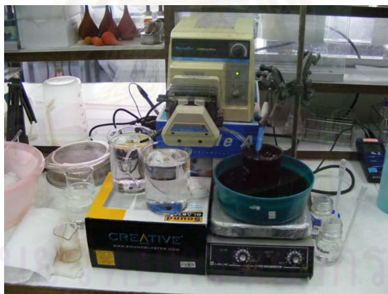
Figure A.2 Fenton experiment in the continuous mode operation for determination of intrinsic rate constant of 2,6-DMA and \text{OH}^\bullet .
