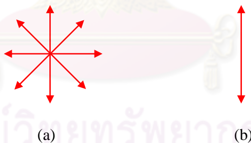
Figure 2.5 (a) an unpolarized light beam viewed along the direction of propagation. The time varying electric field vector can be in any direction in the plane of the page with equal probability. (b) a linearly polarized light beam with the time-varying electric field vector in the vertical direction.
