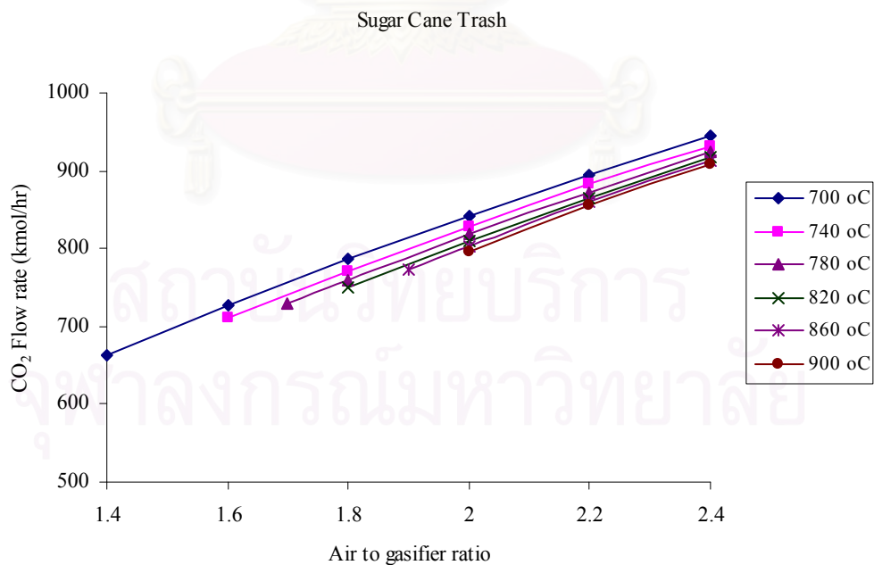
Figure 5.2 Effect of gasifier temperature and air to gasifier ratio to mole flowrate of CO 2 emission for sugar cane trash
