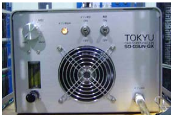
Figure 4.4 Ozone generator model SO-O3UN-OX of Tokyu Car Co., Ltd
