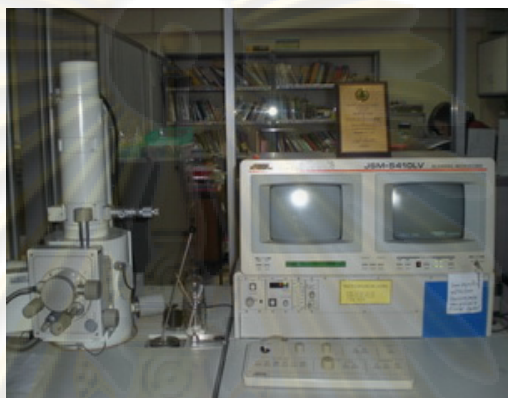
Fig. 3.7 Scanning electron microscope (SEM : Model Jeol JSM-5410LV)
