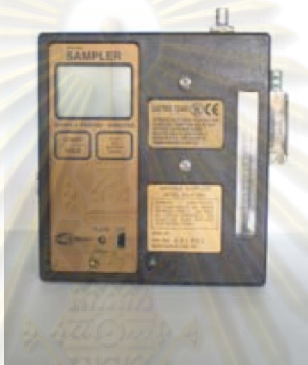
Fig. 3.4 Aerosol personal pump
