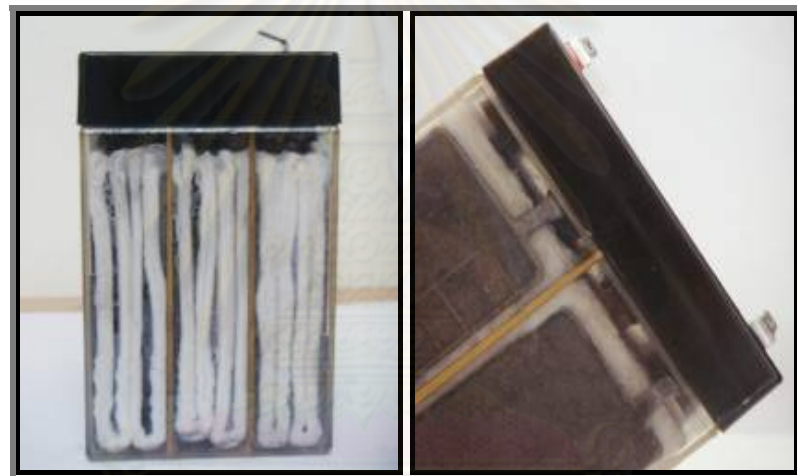
Figure 4.10 A battery filled with electrolyte containing 2% w/v fumed silica and 0.02% w/v PAM in 35% w/v sulfuric acid
