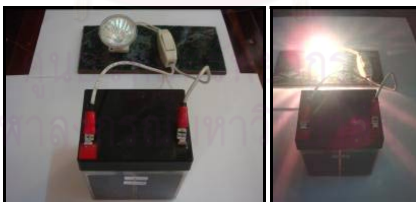
Figure 3.4 Instrument for battery discharging through a 35-Watt helium lamp
