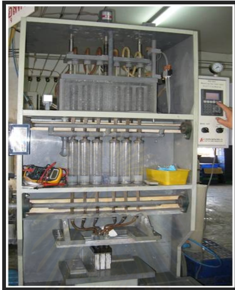
Figure 3.1 Electrolyte filling machine (N.V. Battery Ltd., Thailand)
