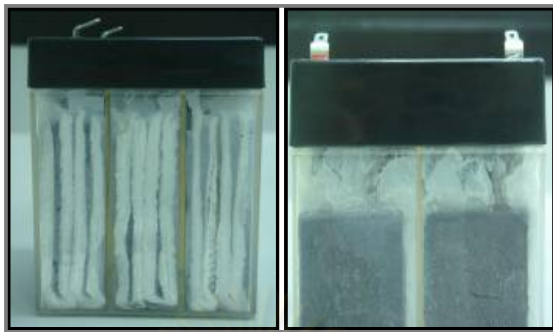
Figure 4.11 A battery filled with electrolyte containing 3%w/v fumed silica and 0.016%w/v PAM in 35%w/v sulfuric acid
