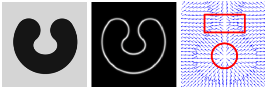
Figure 2.9 (a) a U shape image (b) edge map (c) saddle point (rectangle) and stationary point (circle). (Phumeechanya et al. , 2010)
