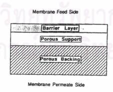
Figure 2.12 Thin-film composite membrane structure (Sirkar and Winston, 1992).
