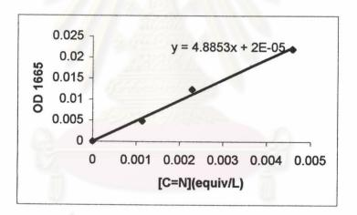
Figure 2.7 Standard curve between the imine concentration ([C=N]) and the imine absorbance at 1665 cm<sup>-1</sup> (OD 1665)
