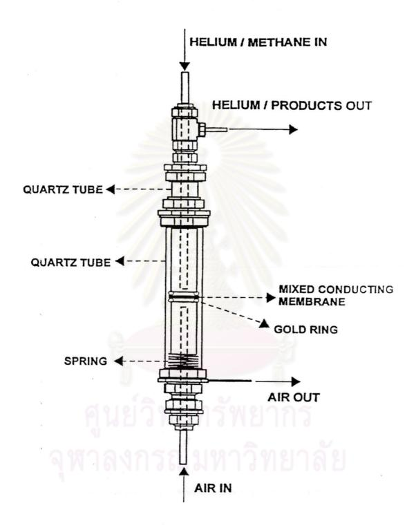
Figure 3.3 A Disc-shaped membrane reactor used in all experiments
