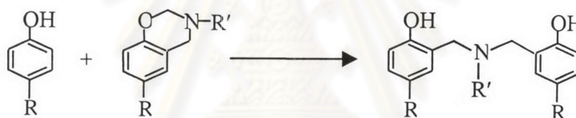
Figure 2.8 Ring-opening reaction of benzoxazine ring with phenolic hydroxyl group.
