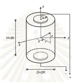
Figure 3.3 A piezoelectric cylinder under applied electric potential.
