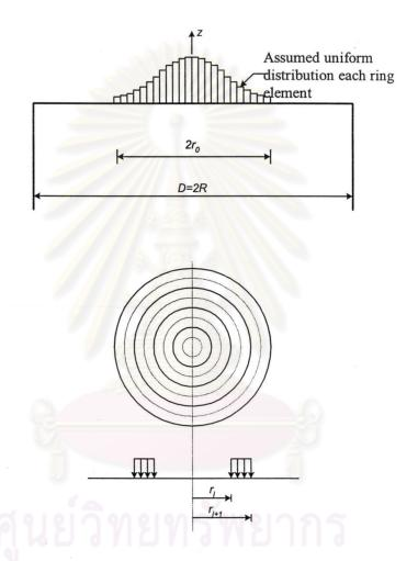
Figure 3.4 Discretization of tractions and electric displacement under electrodes for applied electric field.
