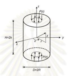
Figure 3.2 A piezoelectric cylinder under applied mechanical loading.
