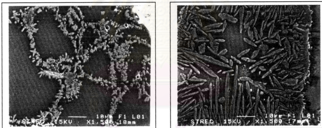
Fig.D-11 SEM micrographs (1500x) of pyroxene phase observed in GC#3 after heat-treatment at condition B (a) C (b)
