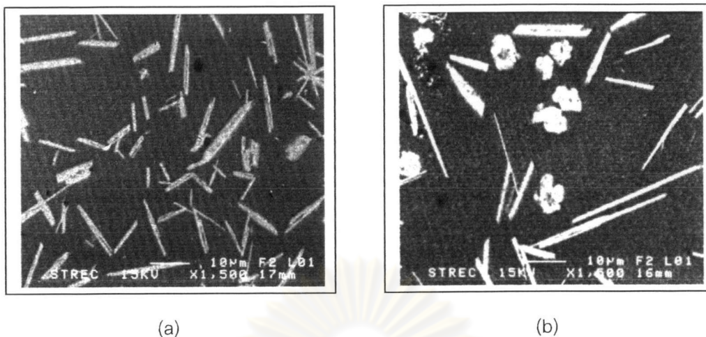
Fig.D-38 SEM micrographs (1500x) of cristobalite, quartz and wollastonite-ferroan phase observed in GC#8 after heat-treatment at condition B (a) C (b)
