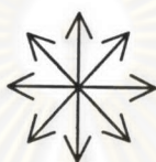
Figure 2.3 Vibrations of electric field vector in unpolarized light
