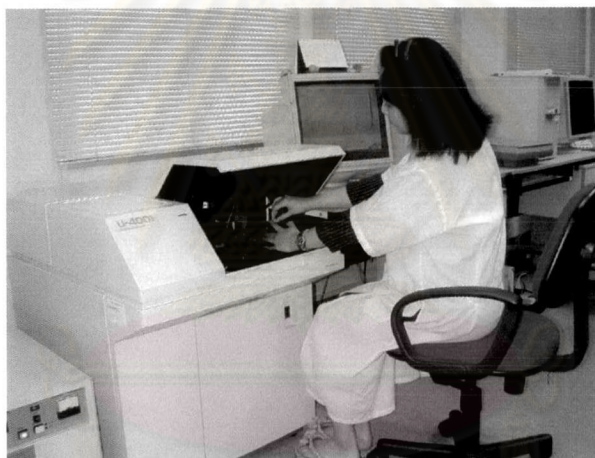
Figure 4.7 UV-VIS-NIR spectrophotometer belonging to the Gem and Jewelry Institute of Thailand (GIT) was engaged for this research.
