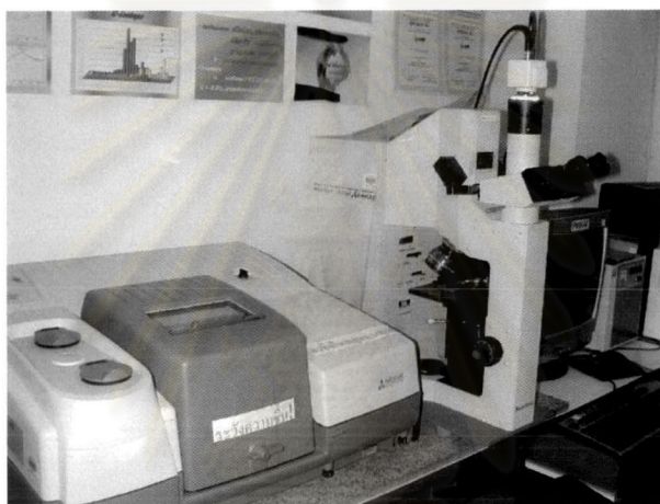
Figure 4.1 Fourier Transform Infrared (FTIR) Spectrometer (NEXUS 470 FT-IR ESP) belonging to Department of General Science, Kasetsart University.
