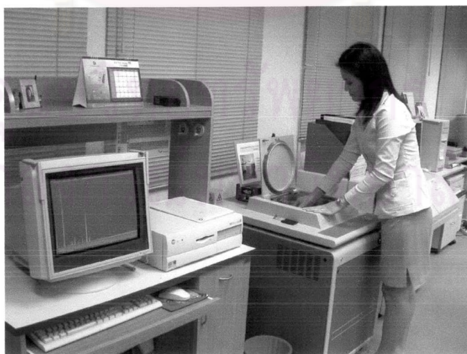
Figure 6.1 Oxford energy dispersive X-ray fluorescence spectrometer, model ED 2000, based at GIT.
