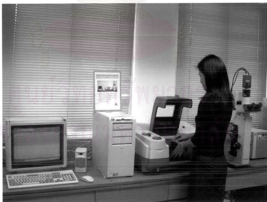
Figure 4.10 Fourier Transform Infrared (FTIR) Spectrophotometer (Nicolet model NEXUS 670 belong to GIT)
