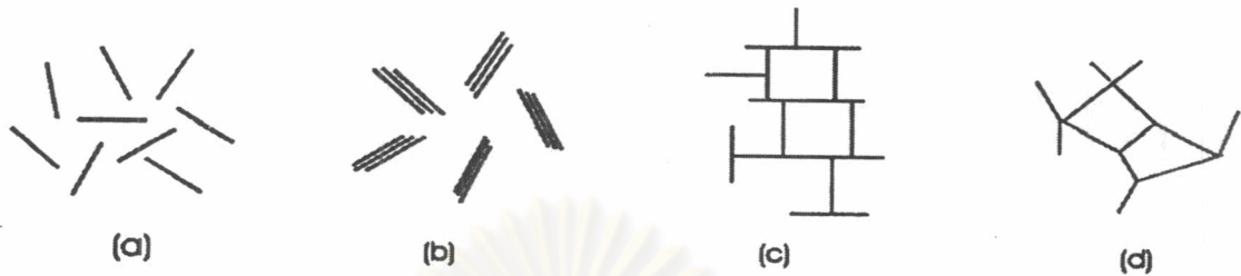
Figure 2.6 Different modes of clay particle association in suspension: (a) dispersed; (b) face-to-face FF; (c) edge-to-face EF; and (d) edge-to-edge EE.
