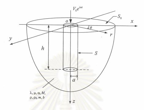
Figure 1.1 Geometry of rigid cylinder embedded in poroelastic half space
