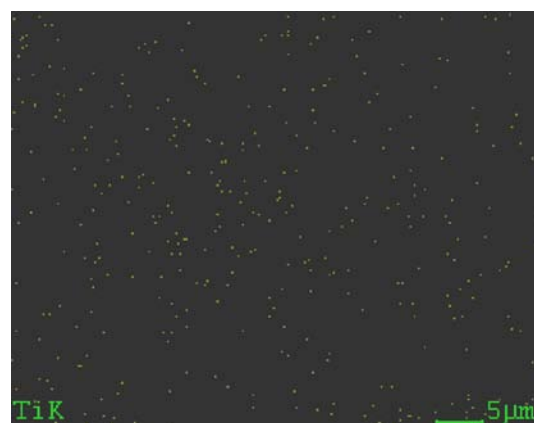
Figure D-1 SEM/EDX of Cat-A under 2000x microscopy
