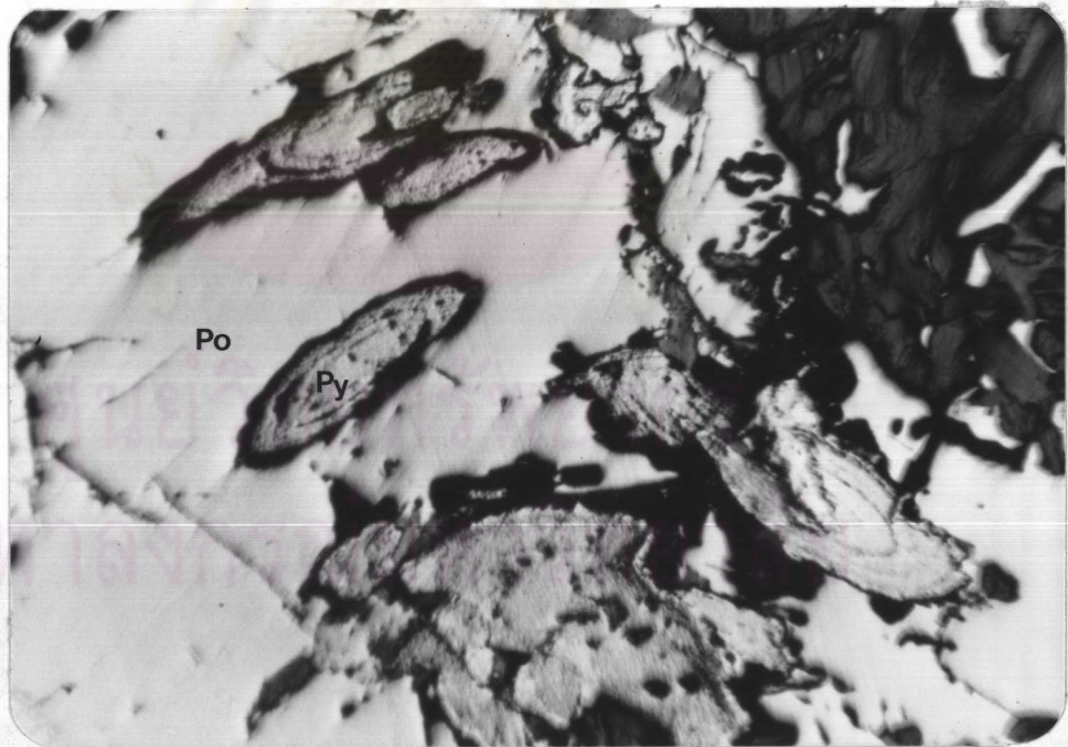
Figure 49 Photomicrograph showing oval shape of pyrite (Py) surrounded by pyrrhotite (Po) filling vugs of marble near the No.1 orebody. (Polished section, 45x, uncrossed nicols)
