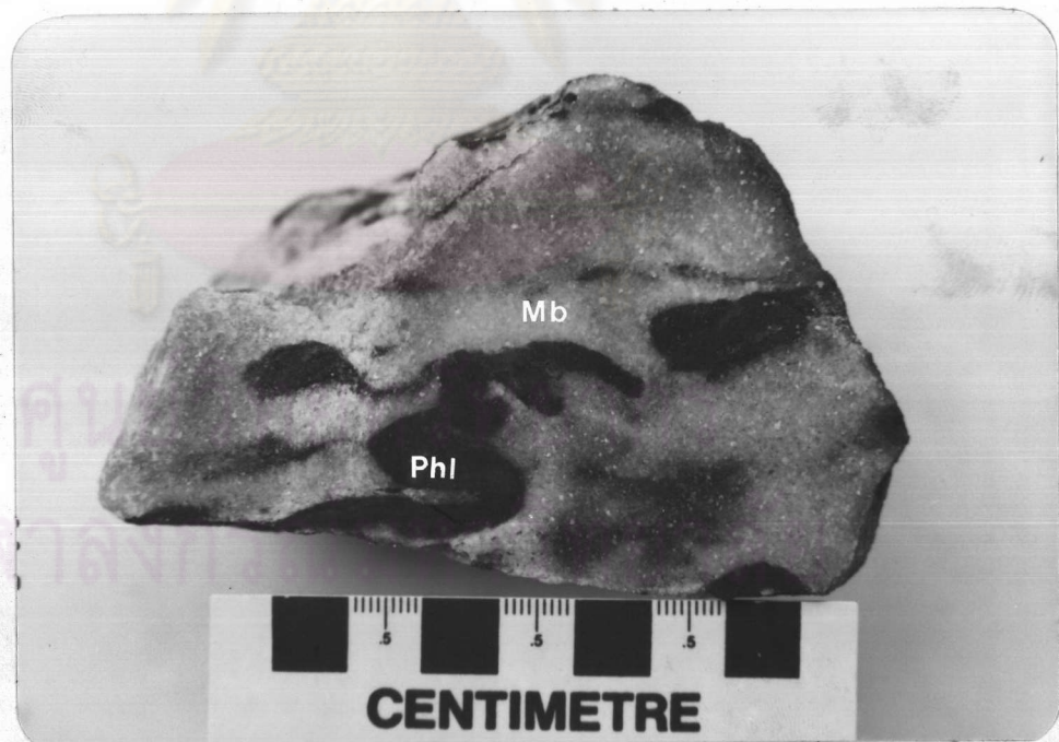
Figure 33 A marble sample showing the distorted patches (Phl) of predominantly phlogopite near the No.1 orebody at the Takua Pit Thong mine.
