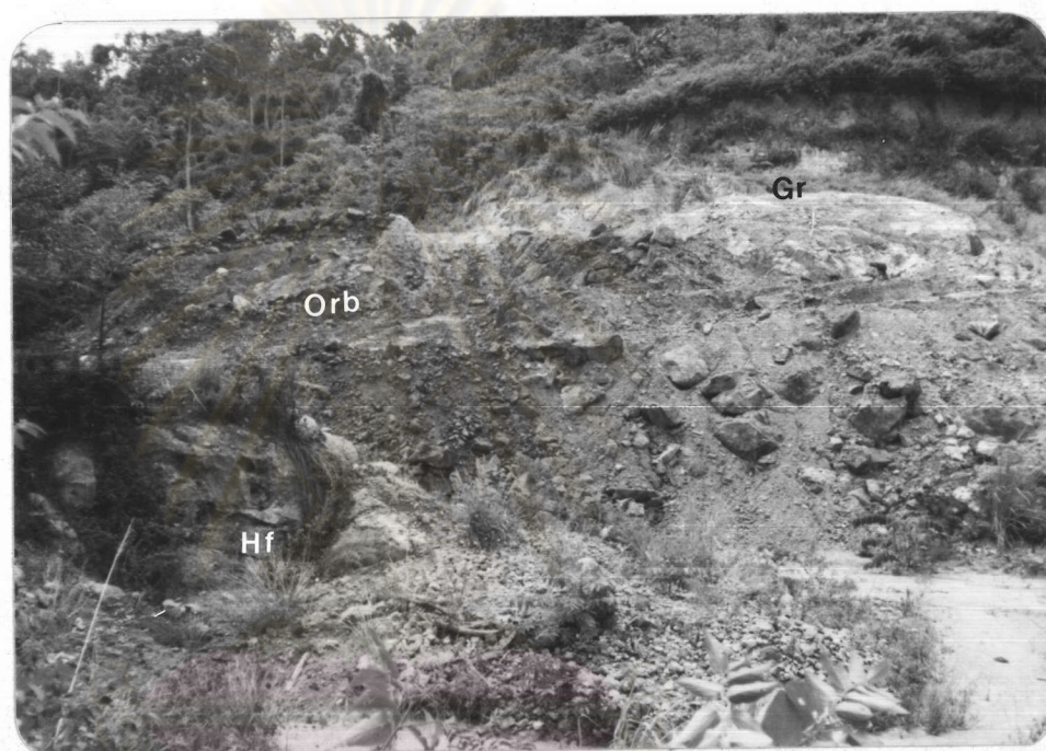
Figure 31 An overview of the No.2 orebody showing outcrop of calcsilicate hornfels (Hf), granitic rocks (Gr) and orebody (Orb).
