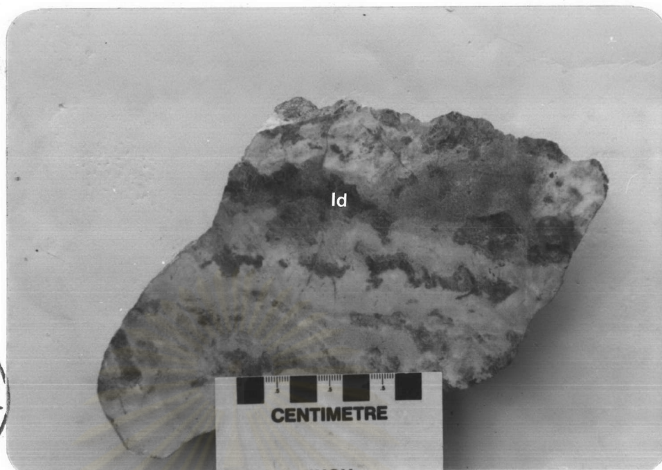
Figure 35 A sample of calcsilicate hornfels near the No.1 orebody showing the development coarse-grained brownish bands (Id) of mainly idocrase at the Takua Pit Thong mine.
