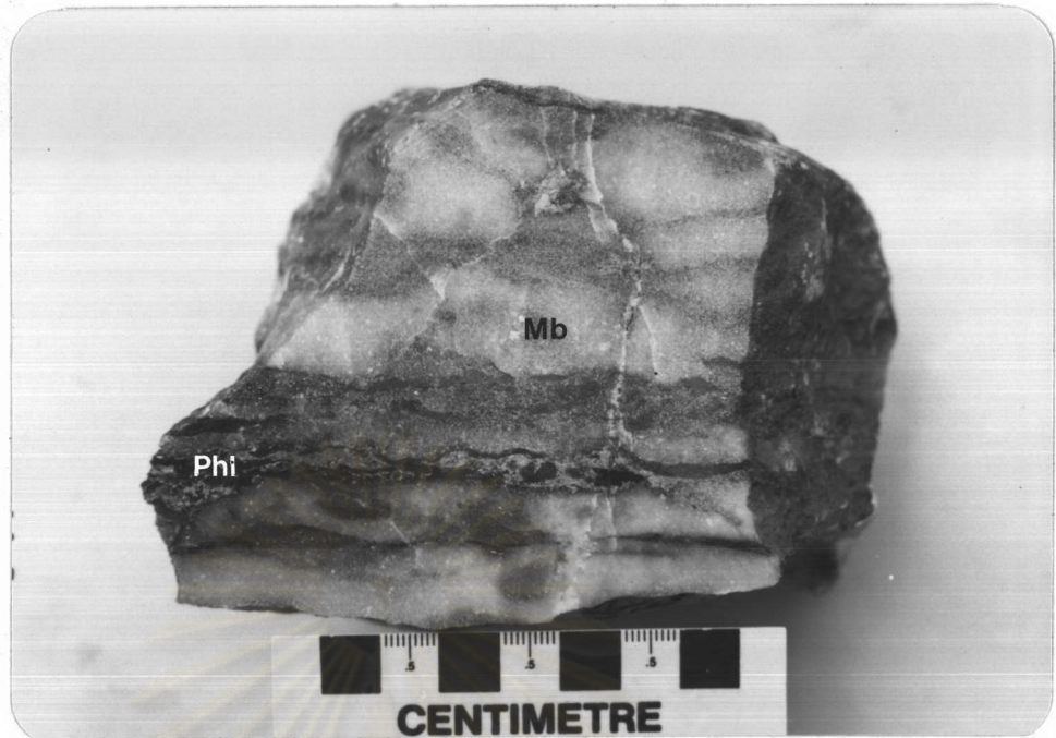
Figure 32 A hand specimen of marble (Mb) near the No.1 orebody. The rock contains dark bands (Phl) of mainly phlogopite and minor sulfide minerals.
