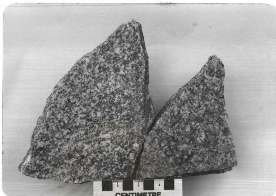
Figure 5 Hand specimens of coarse-grained biotite-muscovite granite at the Takua Pit Thong mine.
