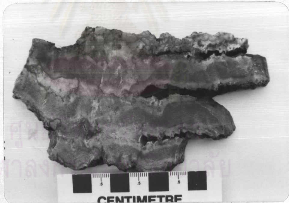
Figure 13 Hand specimen of calcsilicate hornfels at the Takua Pit Thong mine showing bands of original bedding.
