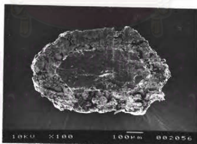
Figure 15 Photomicrographs of coated sucrose beads formulation 4 (Key: A coated beads x 35 , B coating surface x 500 , C cross-section x 100)
