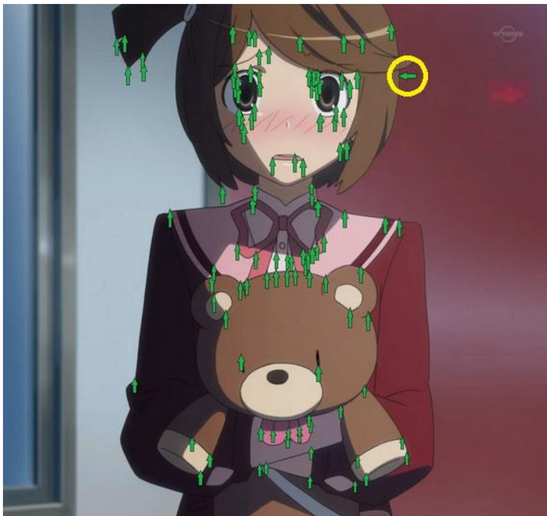
Figure 3.3: Optical flow visualization where the camera is panning downward with some local optical flow circled. ©Tamiki Wakaki/Shogakukan, Kaminomi project, TV TOKYO
